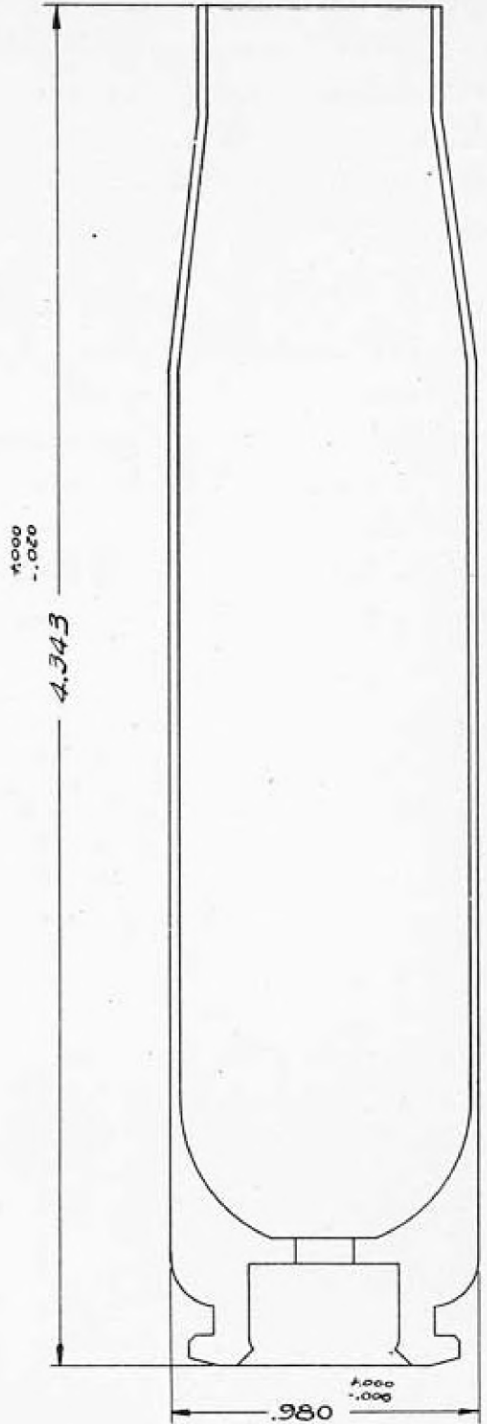
MK.2 20 MM. MK.3 CARTRIDGE CASE
