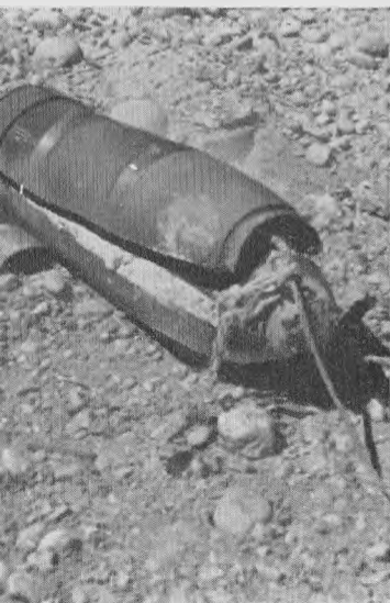
FIGURE 4 Right Below—VT fuze 5" projectile with linear shaped charges wired in place.
