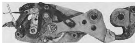
Safety Lever Pulled (Side Plate Removed)
