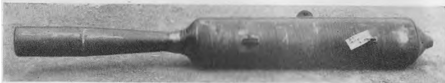
Motor Unit Model 20. Propulsion unit for Baka Bomb.
