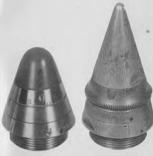
g—Type 0 Mechanical Time Fuze
