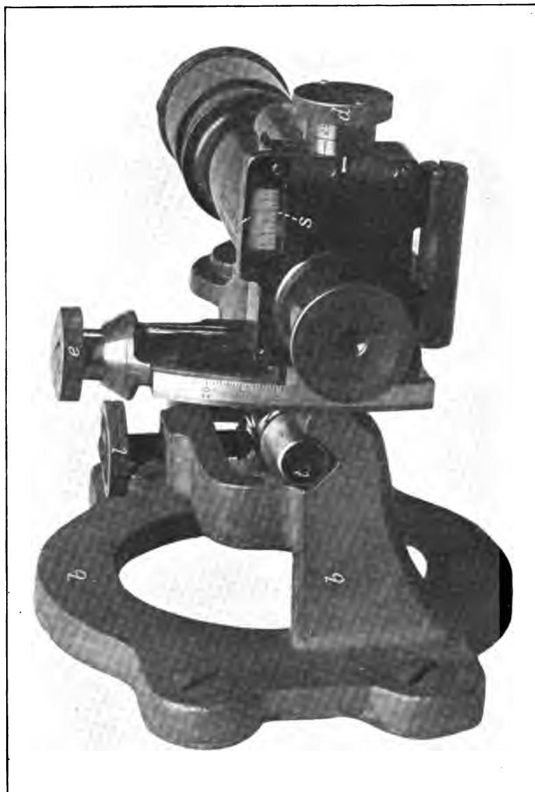
FIG. 260.—Telescopic Sight, Model 1898.
