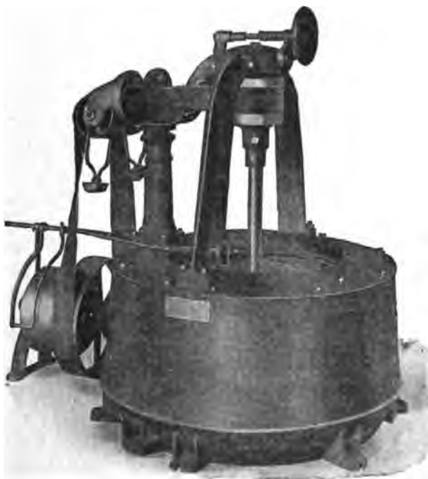
FIG. 8.—Tolhurst Centrifugal Wringer.
