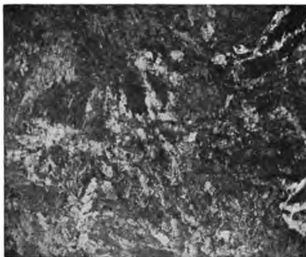
FIG. 50. 0.83% carbon. Practically pure pearlite. Magnification 75.
