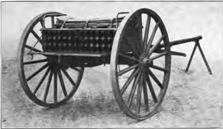
FIG. 164.—3-in. Field Limber.
