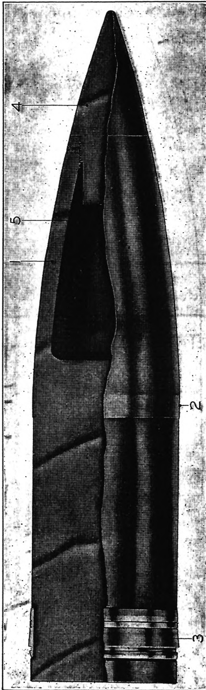
FIG. 8.—Target-practice projectile 1. Cast-iron body. 2. Bourrelet. 3. Rotating band. 4. Nose plug. 5. Empty cavity.
