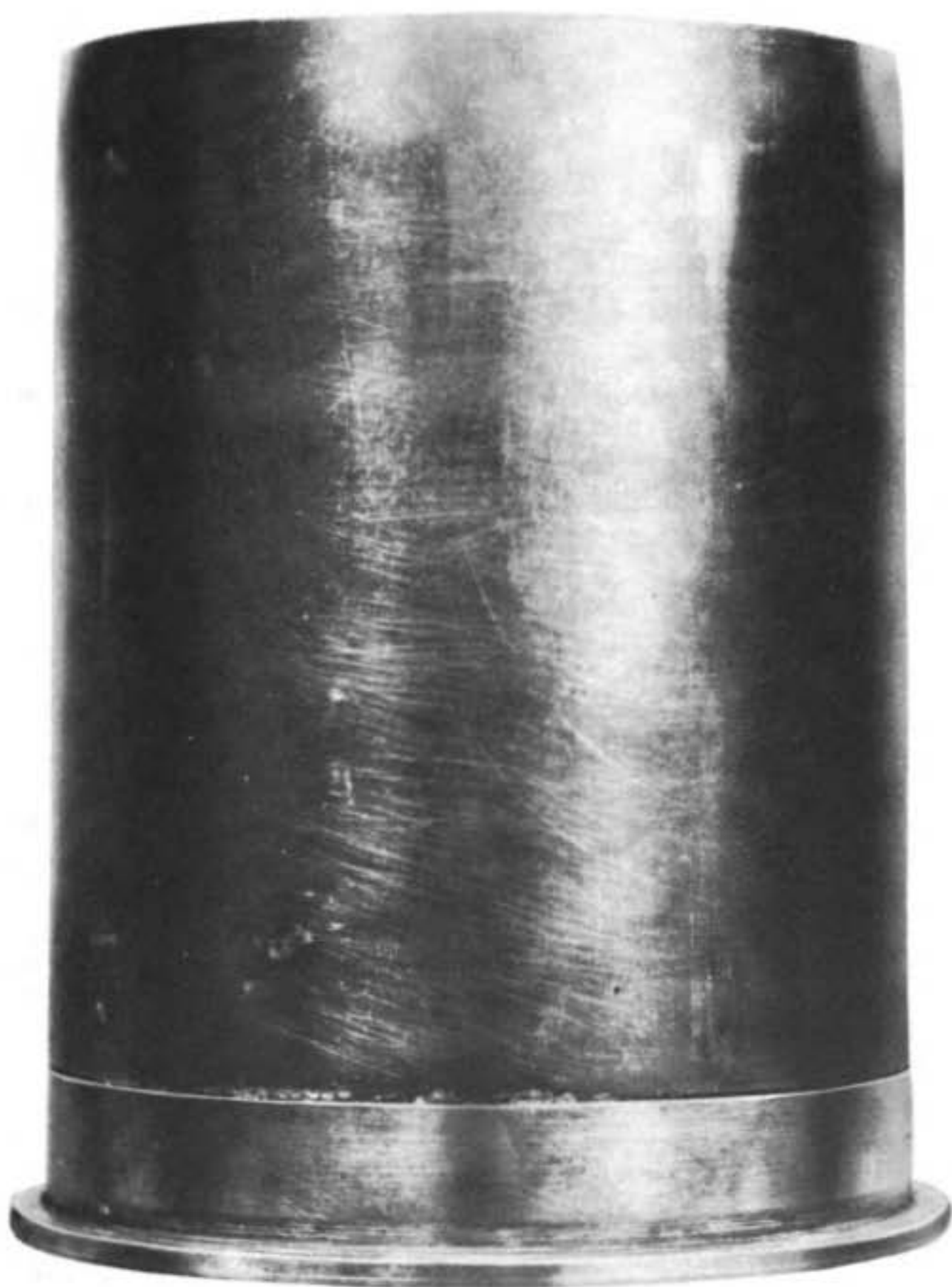
Figure 106—Sectional Type of Cartridge Case for German 105-mm Howitzer
