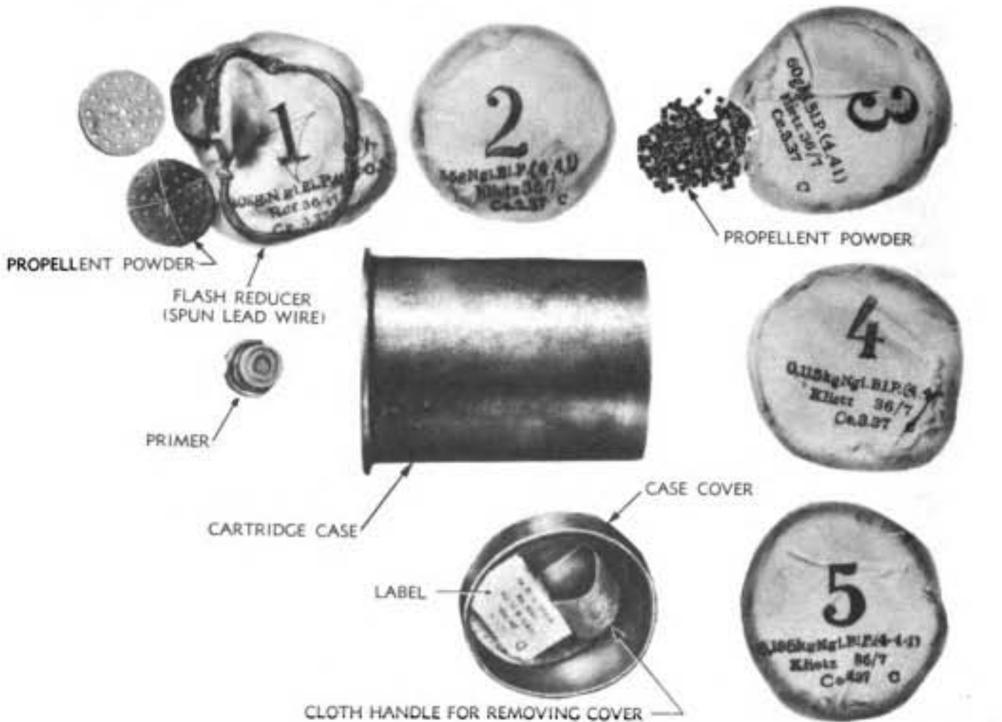
Figure 105—Components of Cartridge Case and Propelling Charge for German 105-mm Howitzer
