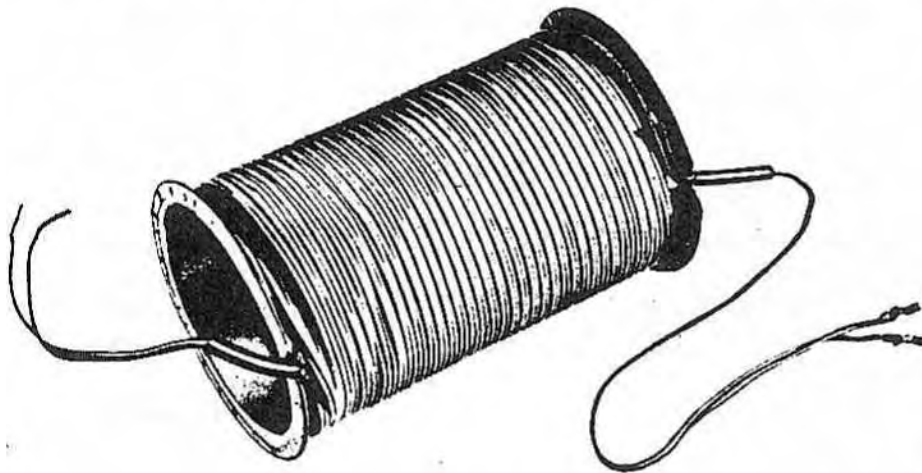
Figure 42—Rear Spacer Tube Wound With Wire
