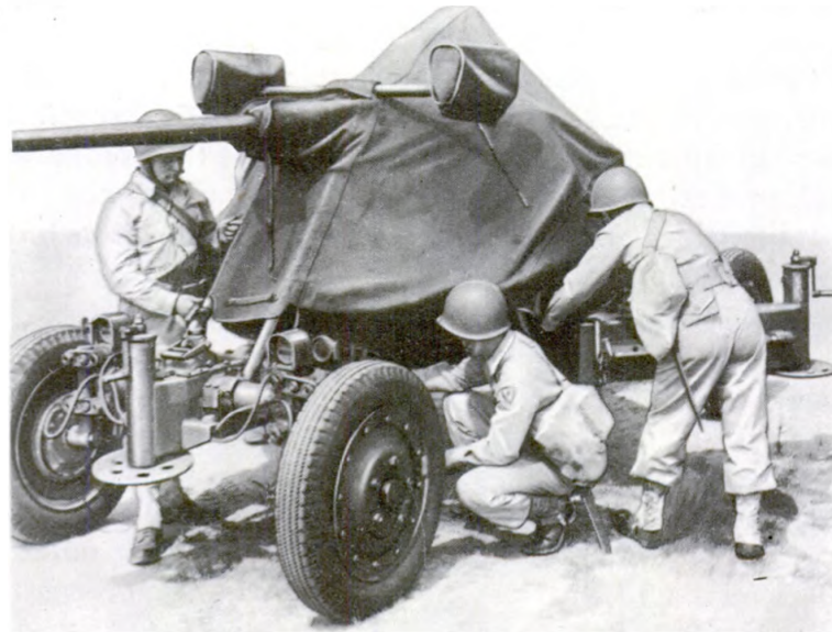
Figure 81 – Removing Outrigger, Carriage, and Sight Covers
