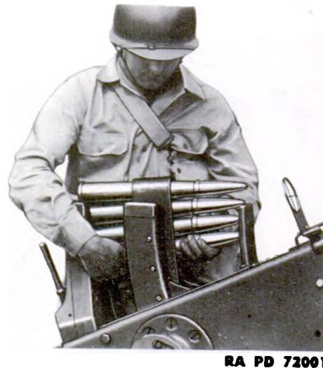
Figure 105 – Removing Cartridges From Automatic Loader
