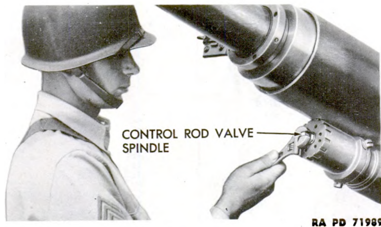
Figure 93 – Adjusting Control Rod Valve
