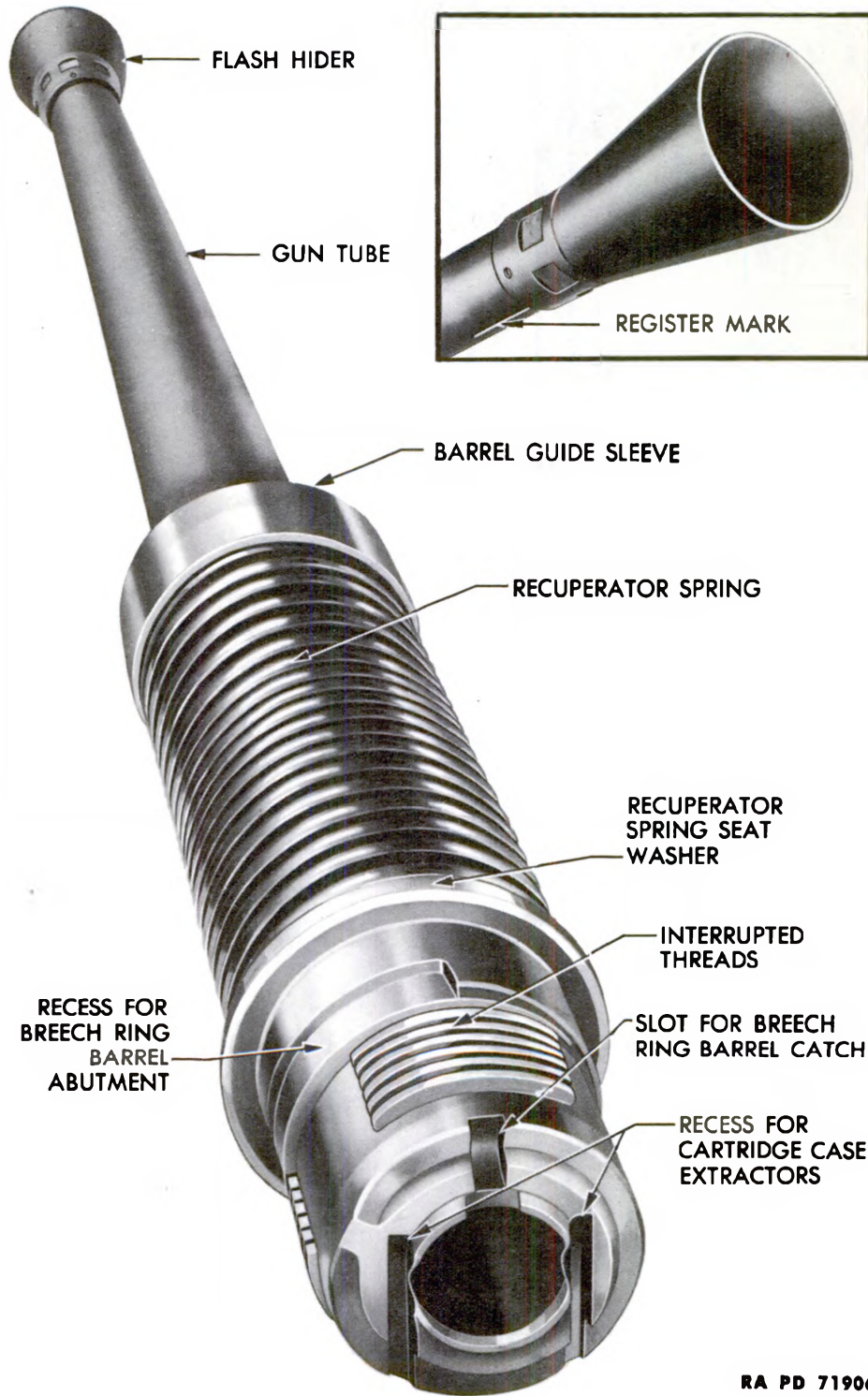
Figure 6 – 40-mm Automatic Gun M1 – Barrel Assembly – Breech End View
