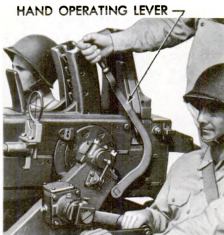
Figure 76 – Opening Breech With Hand Operating lever
