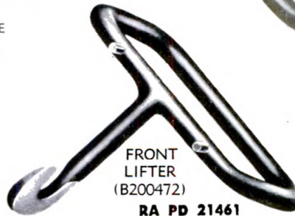
Figure 218 – Front B200472 and Rear B200471 Loader Lifters
