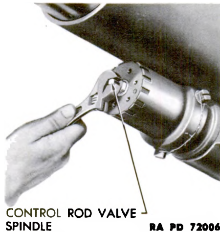
Figure 110 — Adjusting Control Rod Valve Spindle
