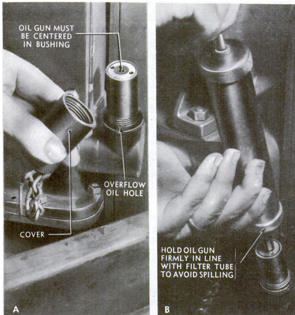
Figure 202 – Pumping Oil Through the Filter of Oil Gear
