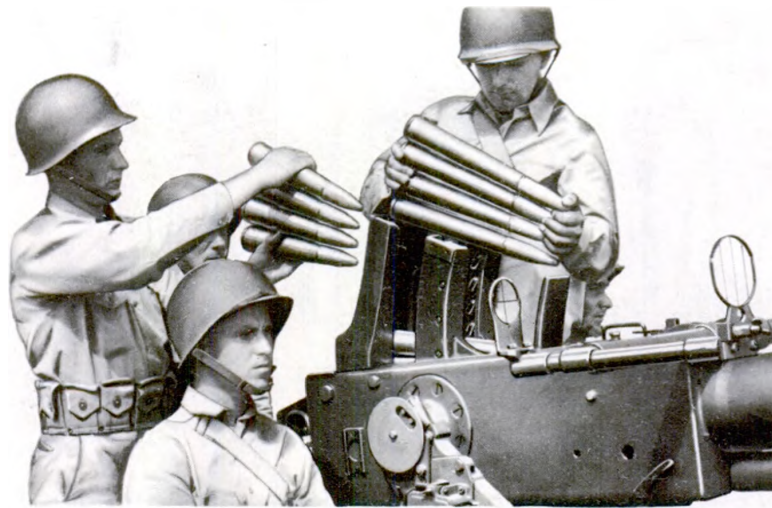
Figure 98 – Inserting Clip Into Automatic Loader
