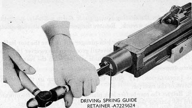
Figure 67. Straightening driving spring guide retainer.
