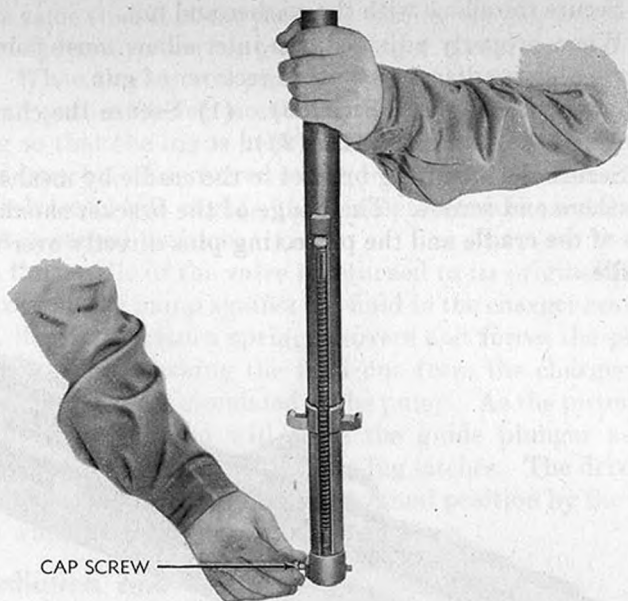
Figure 190. Disassembly of 20-mm hydraulic charger M5.
