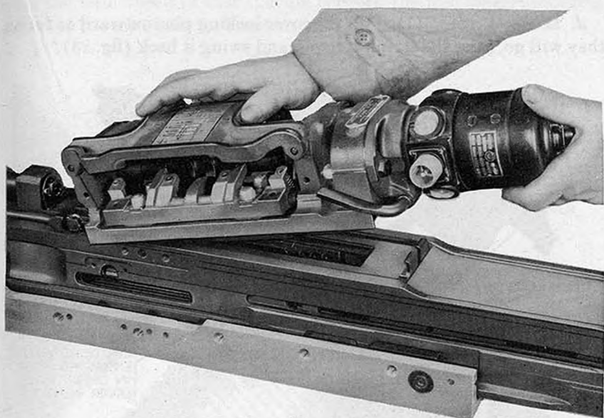
Figure 21. Installing 20-mm feed mechanism M3 on the gun.
