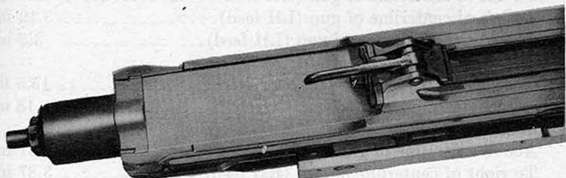
Figure 3. Location of serial number of gun.
