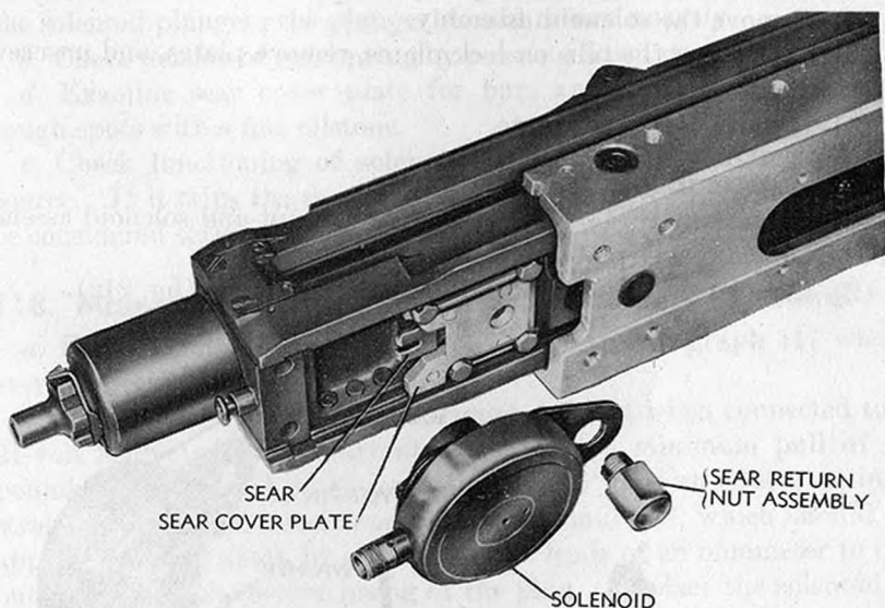
Figure 210. Installing 20-mm electric trigger AN-M4 on gun.
