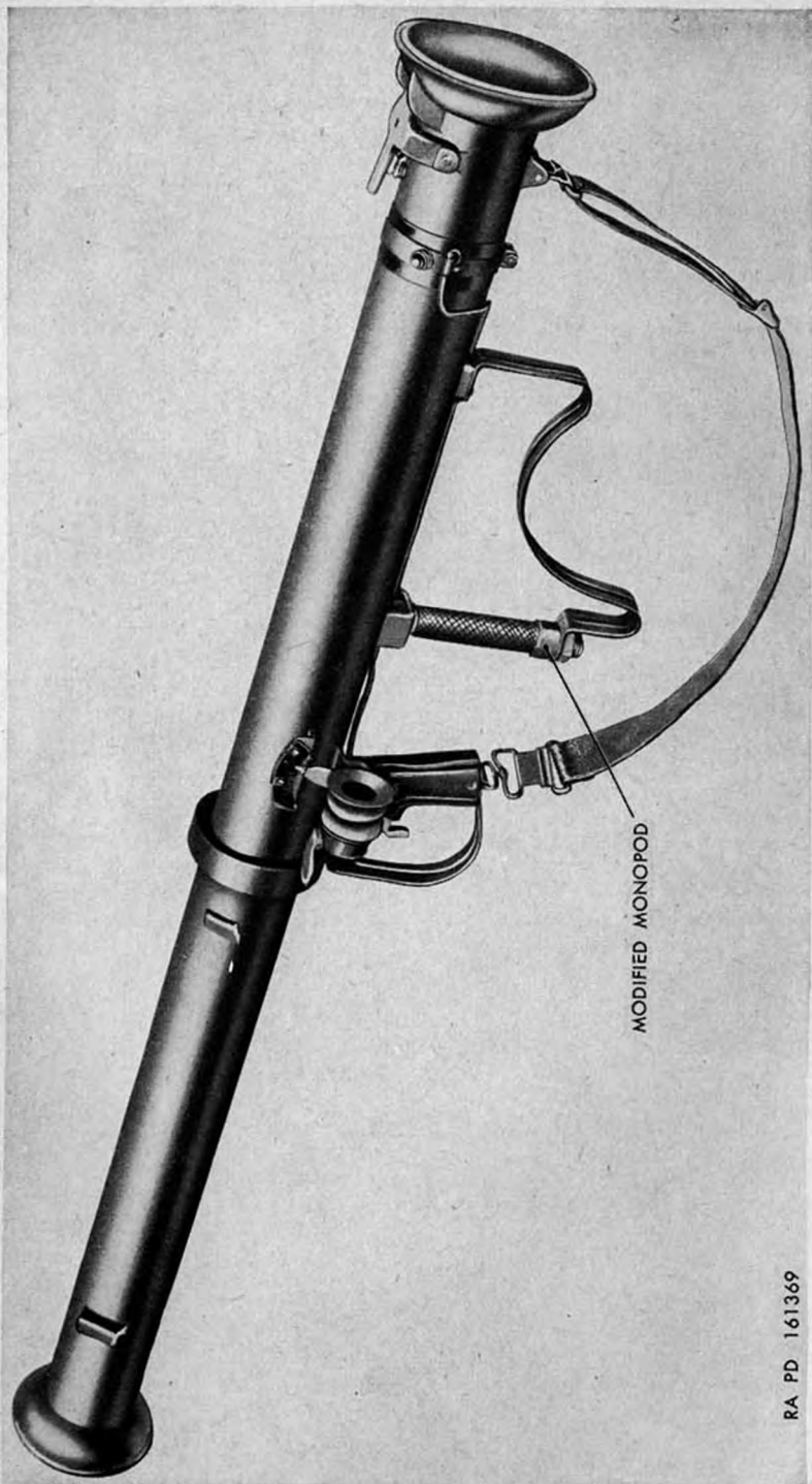
Figure 5. 3.5-inch rocket launcher M20B1 (modified monopod) (early manufacture).
