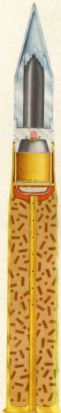
Figure 104. Shot, fixed, HVAP-T, 304, smokeless, for 90-mm guns M1, M1A1, M1A2, M2, M2A1, M3, M3A1, and T8.
