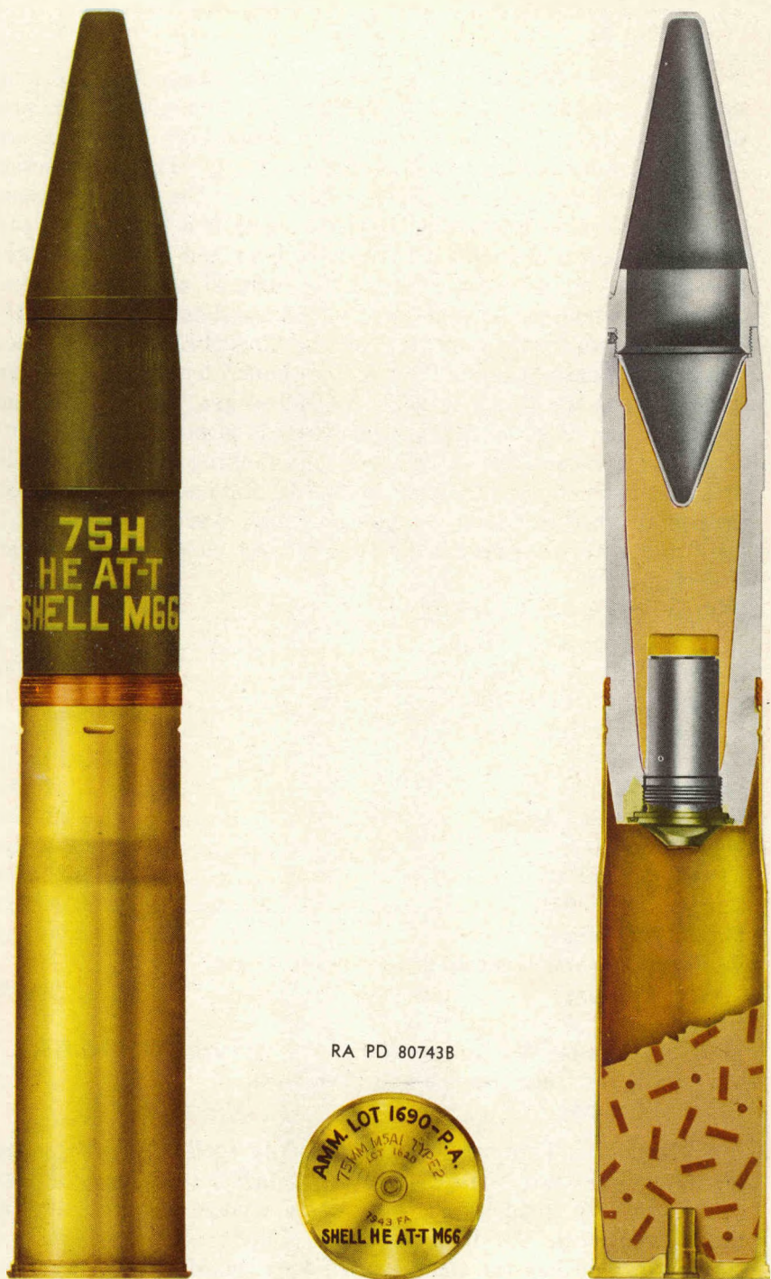
Figure 83. Shell, fixed, HE, AT-T, M66, for 75-mm howitzers.
