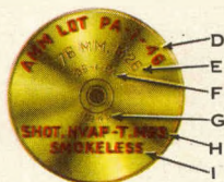
Figure 12. Typical marking of HVAP-T rounds.
