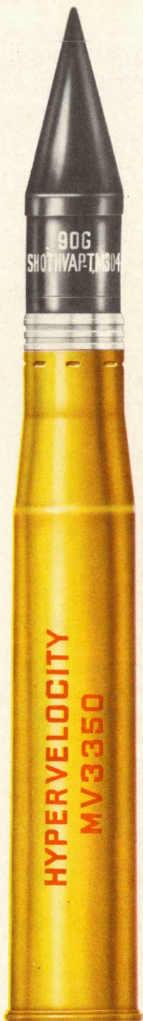
Figure 104. Shot, fixed, HVAP-T, 304, smokeless, for 90-mm guns M1, M1A1, M1A2, M2, M2A1, M3, M3A1, and T8.
