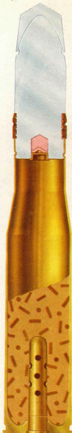
Figure 44. Shot, fired, APC-T, M59A1, for 37-mm guns M1A2 and AN-M9.
