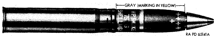
Figure 76. Shell, fixed, smoke, WP, M64, w/fuze, PD, M48A2, 0.05-sec delay, for 75-mm guns.
