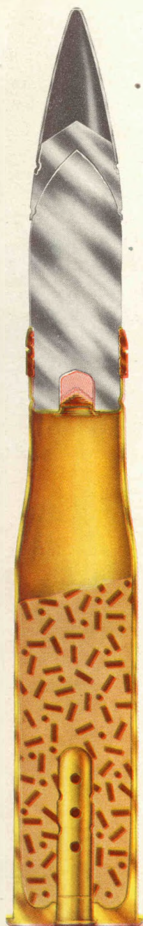
Figure 47. Shot, fixed, APC-T, M51, MV 2,900, for 37-mm gun M6.
