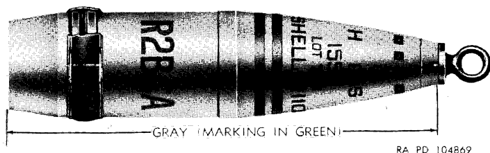
Figure 129. Shell, gas, persistent, H, M110, for 155-mm howitzers.
