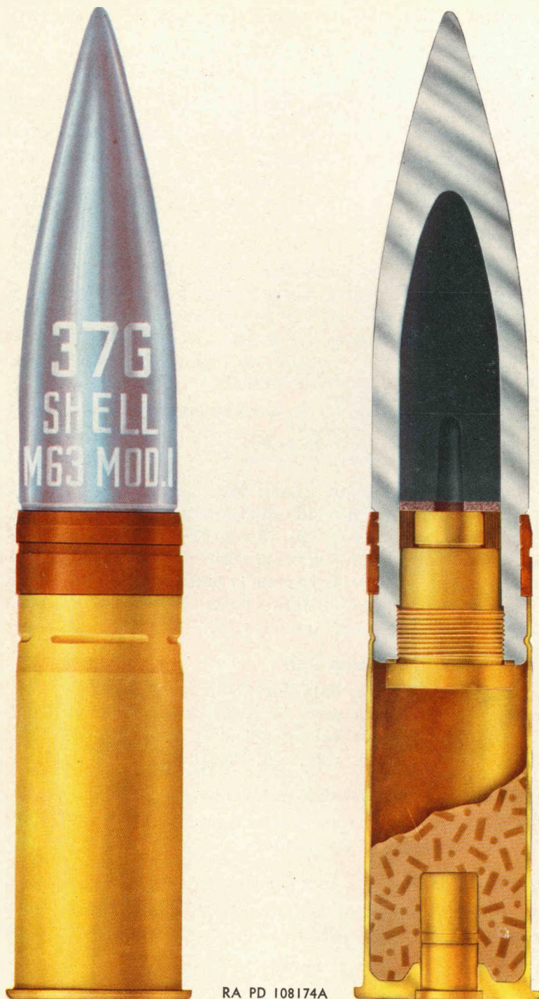
Figure 139. Shell, fixed, TP, M63 mod 1, for 37-mm subcaliber guns.
