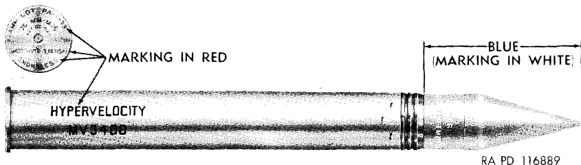
Figure 94. Shot, fixed, HVTP-T, M315A1, smokeless, for 76-mm guns.
