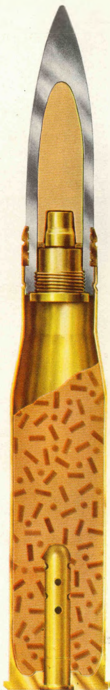
Figure 46. Shell, fixed, HE, M63, w/fuze, BD, M58, for 37-mm gun M6.
