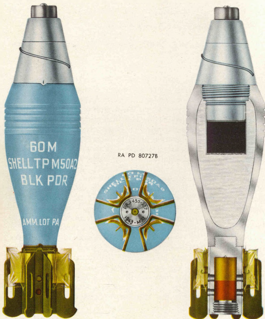
Figure 72. Shell, TP, M50A2, w/fuze, PD, M52A1, for 60-mm mortars.
