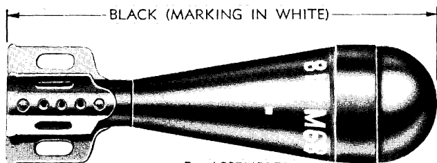
Figure 102. Shell, training, M68, w/o fin assembly, for 81-mm mortars.
