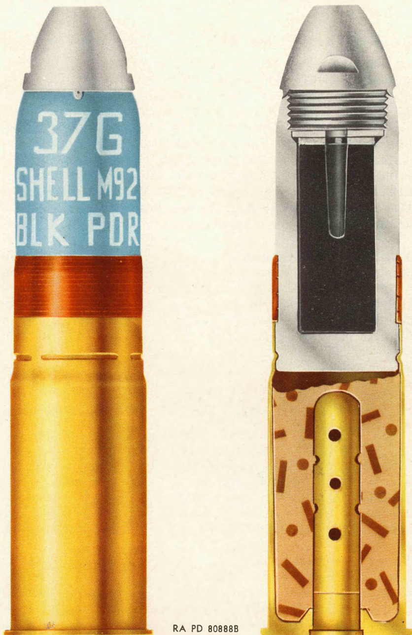
Figure 140. Shell, fixed, TP, M92, w/fuze, PD, M74, for 37-mm subcaliber guns.
