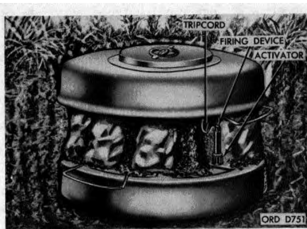
Figure 7-13. Installation of a boobytrapped AT mine.
