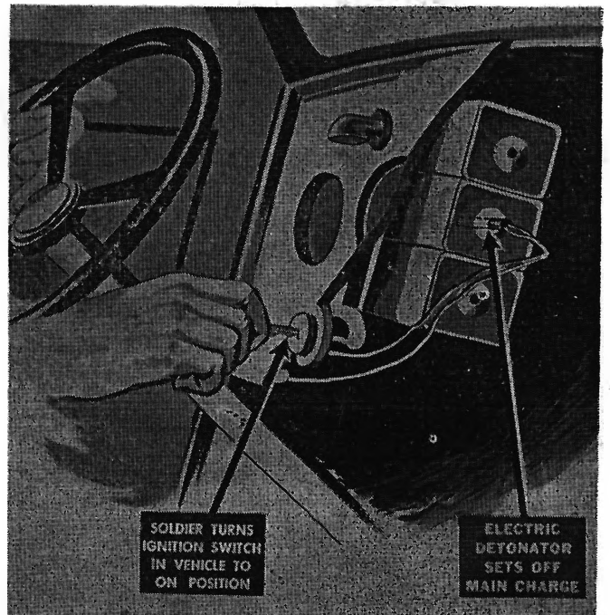
Figure 12. Ignition by electrical means.
