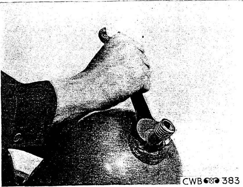
FIGURE 20.—Burster-tube assembly screwed into shell and tightened with wrench.
