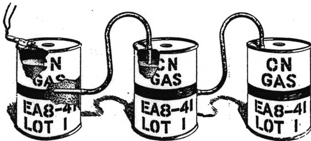
FIGURE 10.—CN tear gas pots—sectional diagram, electrical firing.
