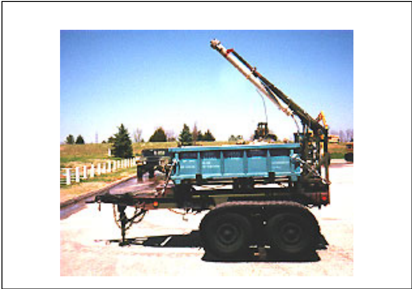
Figure 14-4. Armored Vehicle Launched- Mine Clearing Line Charge
