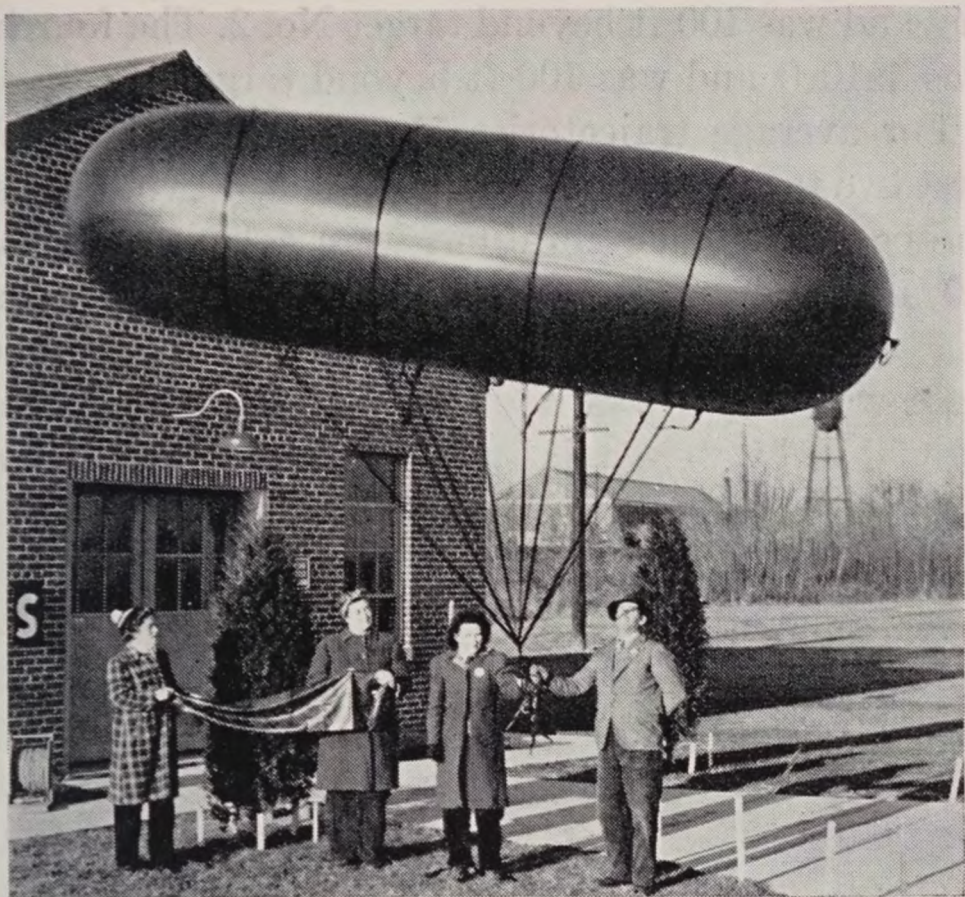
FIGURE 1. Target balloon for plane-firing tests.
