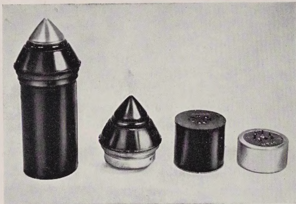
FIGURE 2. T-4 photoelectric fuze, developed for use on M-8 rocket. From left to right are shown: assembled fuze ready for installation in rocket; MC-380 nose containing electronic control elements; BA-75 battery; and SW-230 switch. Nose and switch plug into opposite ends of battery.
