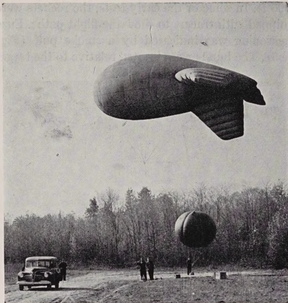
FIGURE 3. Barrage balloon and 12-ft diameter spherical target balloon for photoelectric rocket fuze tests.
