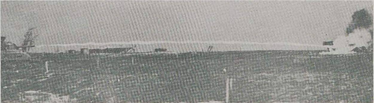
The E12-7R1 firing 8 percent Napalm-thickened fuel at 65 yards.
