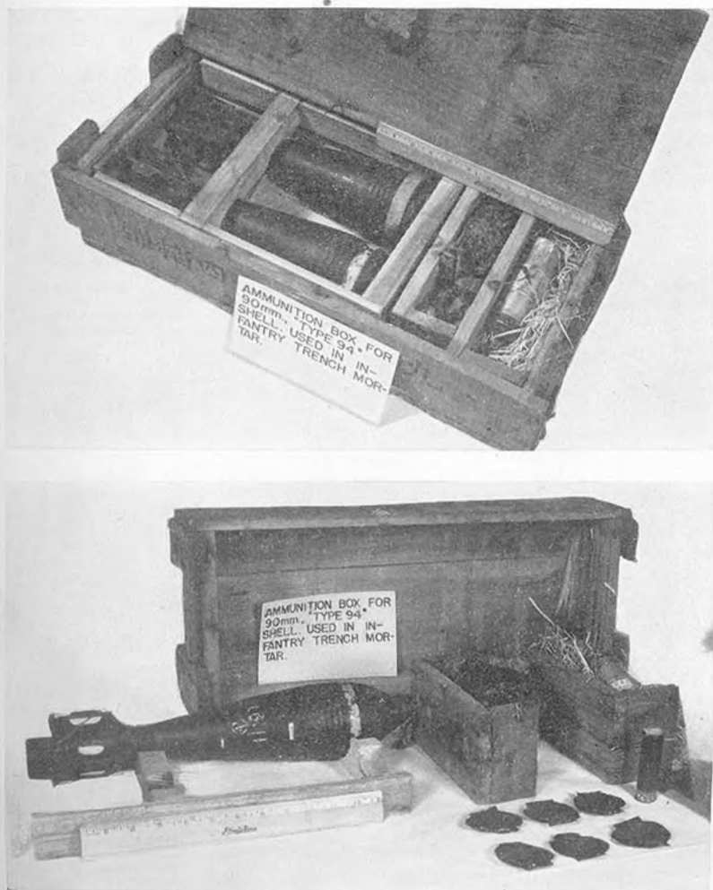
Figure 103.—Model 94 (1934) 90-mm mortar shell with two views of its packing box (two complete rounds).
