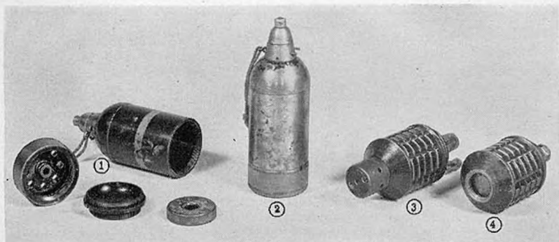
Figure 50.—Two types of ammunition fired in Model 89 (1929) 50-mm grenade discharger. (From left to right are shown the Model 89 (1929) shell ① disassembled, ② assembled; the Model 91 (1931) hand grenade ③ with propellant container, ④ without propellant container.)
