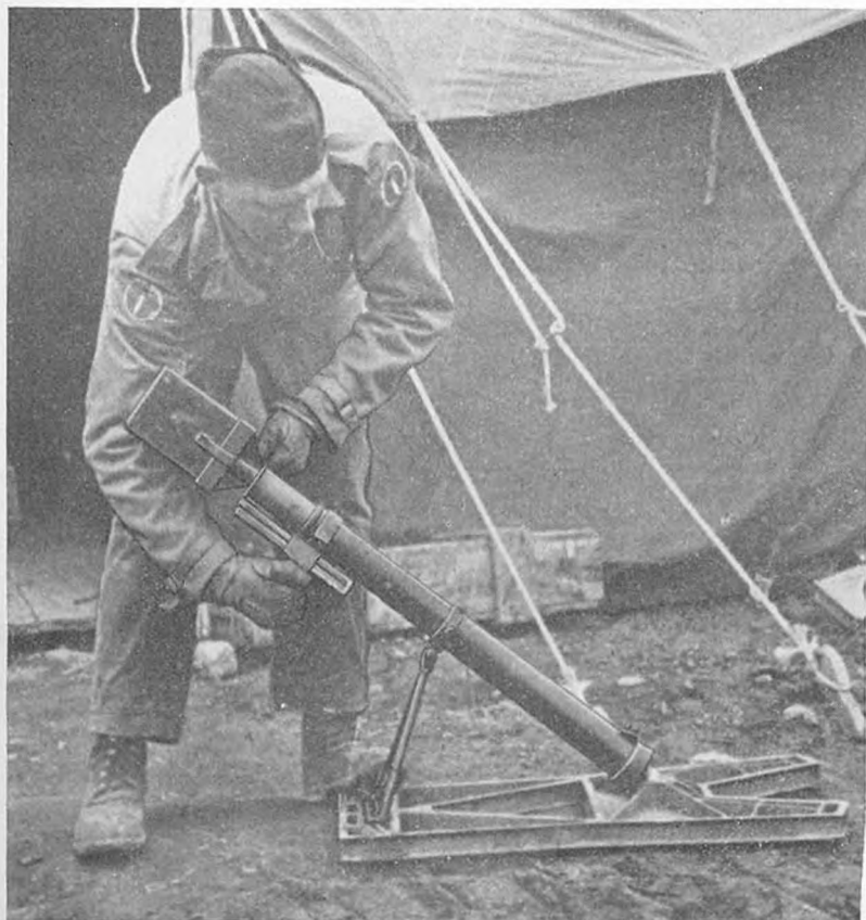
Figure 84.—Adjusting graduated range slide on Model 98 (1938) 50-mm mortar.
