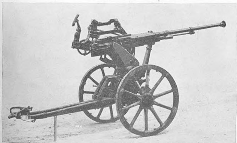
Figure 110.—Model 98 (1938) 20-mm antiaircraft-antitank machine cannon in traveling position.
