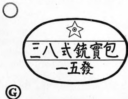
Figure 154.—Label and markings used on box of Model 38 (1905) 6.5-mm semirimmed, reduced-charge ball ammunition. (The markings on the label are read, from left to right, Sampachi Shiki Ju Jippo—Jugo Hatsu , meaning "38 model rifle ball ammunition—15 rounds." © in the lower left corner indicates reduced-charge ammunition. The circle in the upper left corner (which is colored pink) indicates ball ammunition.)
