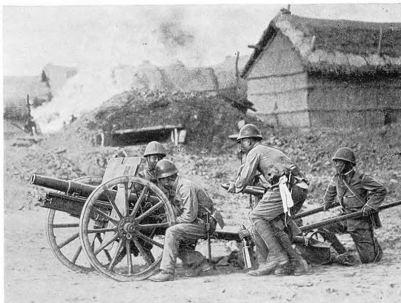
Figure 147.—Gun crew of Model 41 (1908) 75-mm mountain (infantry) gun in action. (Note the method of moving the trail.)
