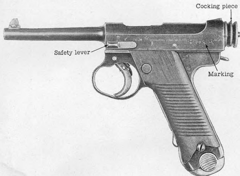
Figure 8.—Model 14 (1925) 8-mm pistol (left side).
