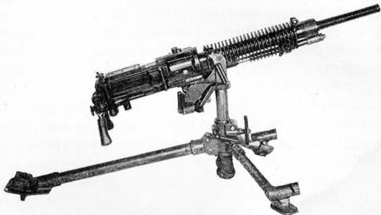
Figure 68.—Model 92 (1932) 7.7-mm heavy machine gun (right side).
