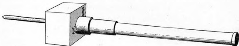
Figure 90. —70-mm barrage mortar, showing spike and block used as balance.
