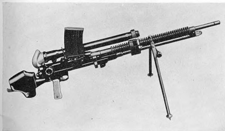
Figure 159.—Model 97 (1937) 7.7-mm tank machine gun on ground mount.
