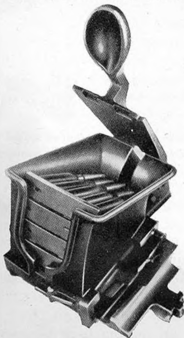
Figure 58.—Loaded feed hopper of Model 11 (1922) 6.5-mm light machine gun.
