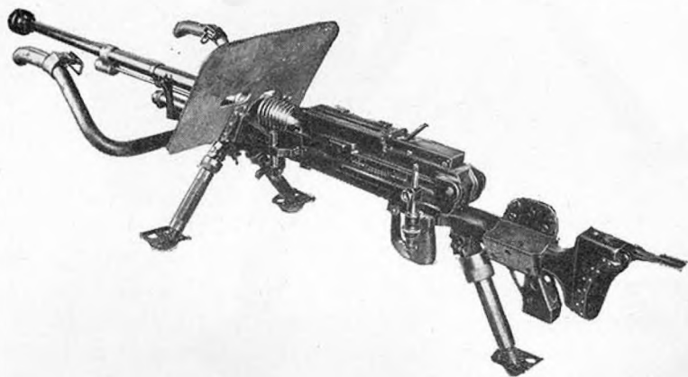
Figure 108.—Model 97 (1937) 20-mm antitank rifle with shield and front carrying handles in place.
