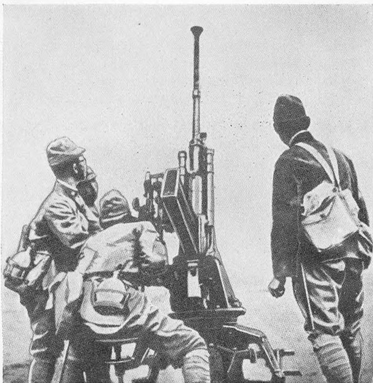
Figure 111.—Model 98 (1938) 20-mm anti-aircraft-antitank machine cannon in action.
