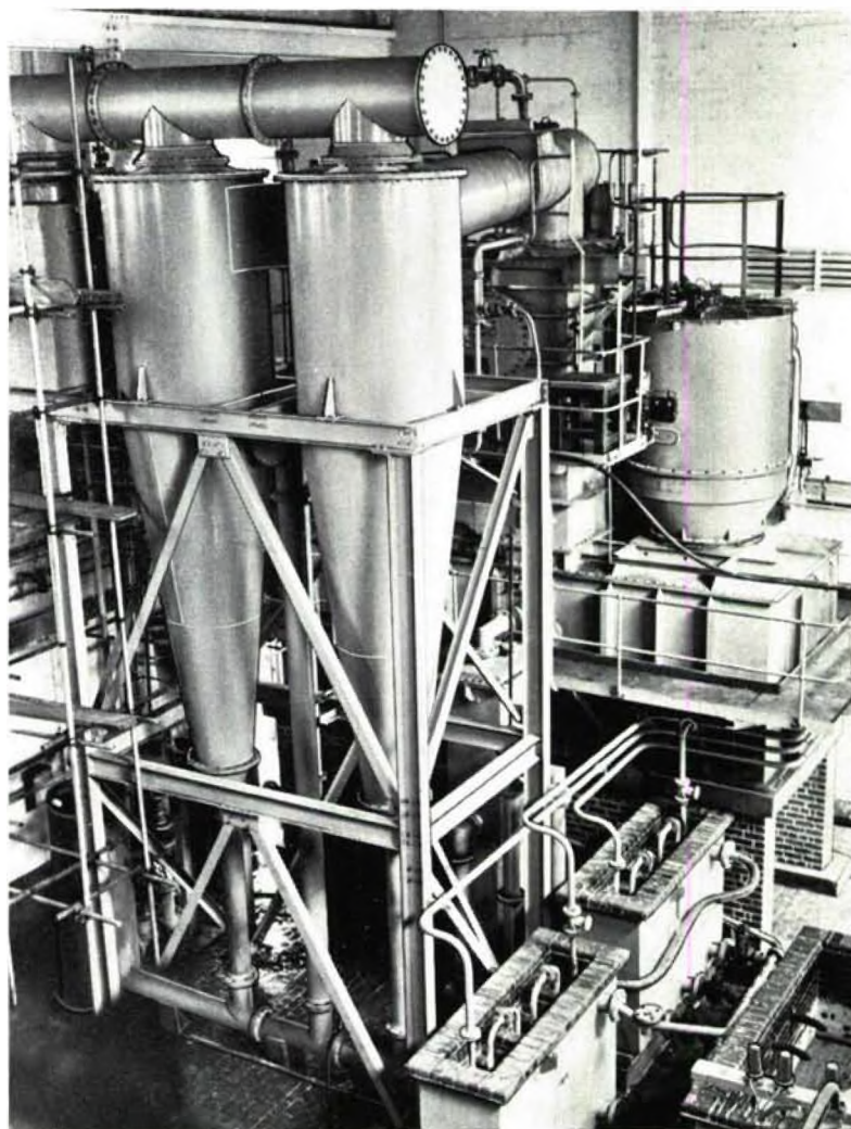
Fig. 2 Concentration of sulphuric acid by submerged combustion
