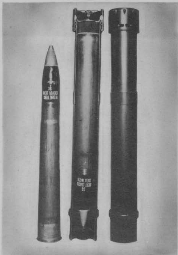
3-inch Metal Container, M158
