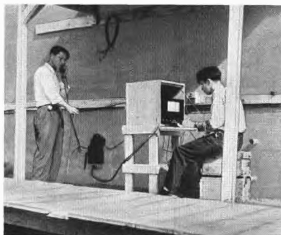
FIGURE 42. Electronic timing device for measuring muzzle velocity.
