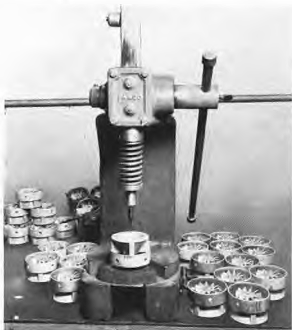
FIGURE 21. Arbor press for staking windmill bearing assemblies.
