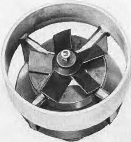
FIGURE 50. Windmill for speed regulation. Normal position of windmill on its shaft (top); windmill depressed by air pressure (bottom).
