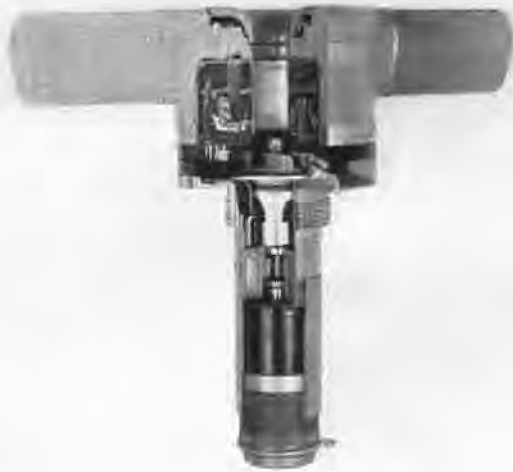
FIGURE 58. Fuze T-82 with section cut away. Central air duct to turbine can be seen. Generator was immediately below and directly coupled to turbine.
