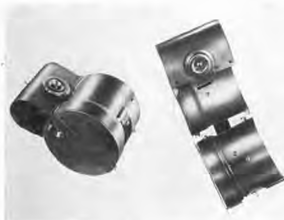
FIGURE 2. Alternative arming delay. This delay completely encloses nose of fuze, preventing air stream from reaching vanes. When it operates, it opens and flies off fuze as shown in picture at right.
