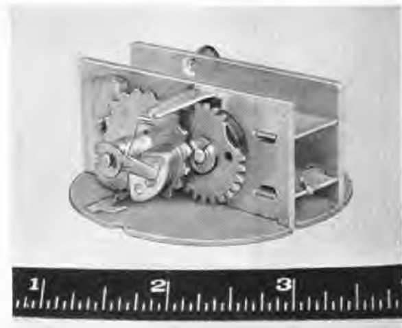
FIGURE 10. Self-destruction element for T-5 fuze.
