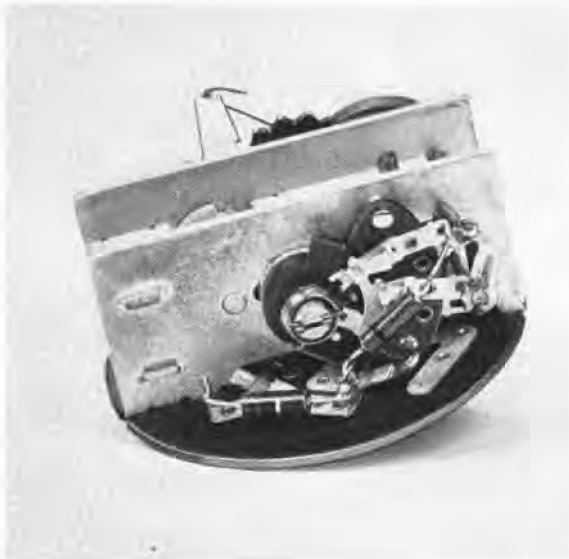
FIGURE 11. Impact detonator for T-6 fuze.
