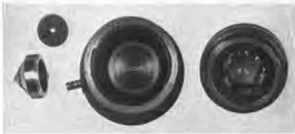
FIGURE 17. Ultra centrifuge for testing rotors for T-50 type fuzes.
