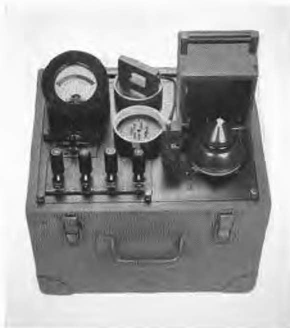
FIGURE 19. Field test set IE-28 with T-4 fuze in position for testing.
