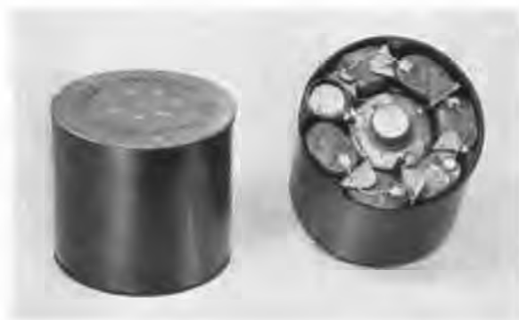
FIGURE 54. Battery pack, BA-75. At left is complete unit. At right is similar unit with end plate removed. Six stacks of layer built cells for B and C voltage, two cylindrical A cells, and detonator firing capacitor can be seen.
