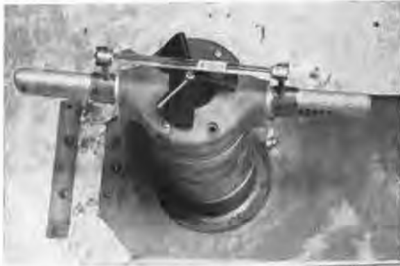
FIGURE 7. Resistor for determining sensitivity of bar-type fuzes.
