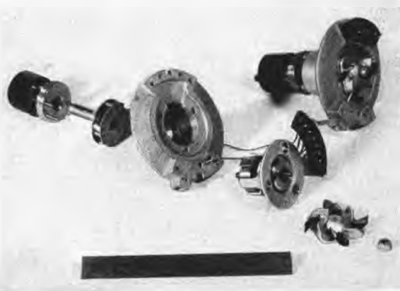
FIGURE 23. Power supply and arming system for T-82 fuzes.
