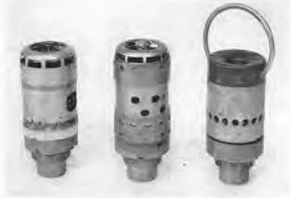
FIGURE 6. Radio proximity fuzes for trench mortar shells. These are, from left to right: (1) T-132 fuze using electric circuits "printed" on ceramic plates; (2) T-171 fuze, electrically similar to T-132 but with standard electrical resistor and condensers; and (3) T-172 fuze with loop antenna.
