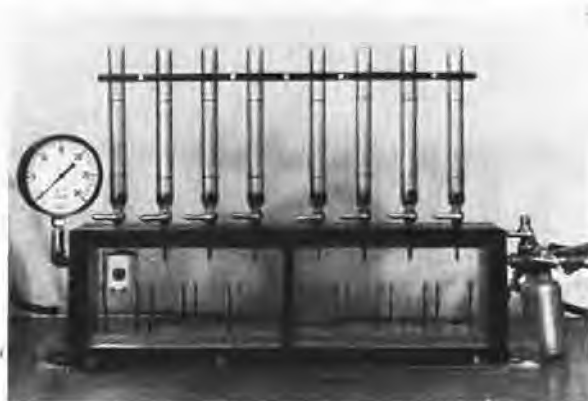
FIGURE 20. Vacuum fixture for potting amplifier units (Globe-Union, Inc., photograph).
