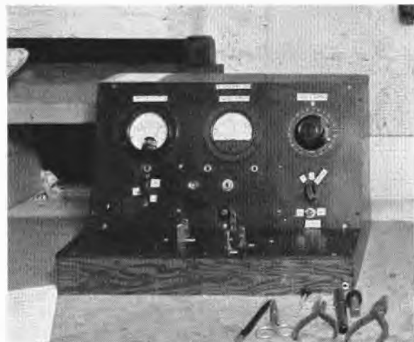
FIGURE 31. Rectifier filter test position (Bowen).
