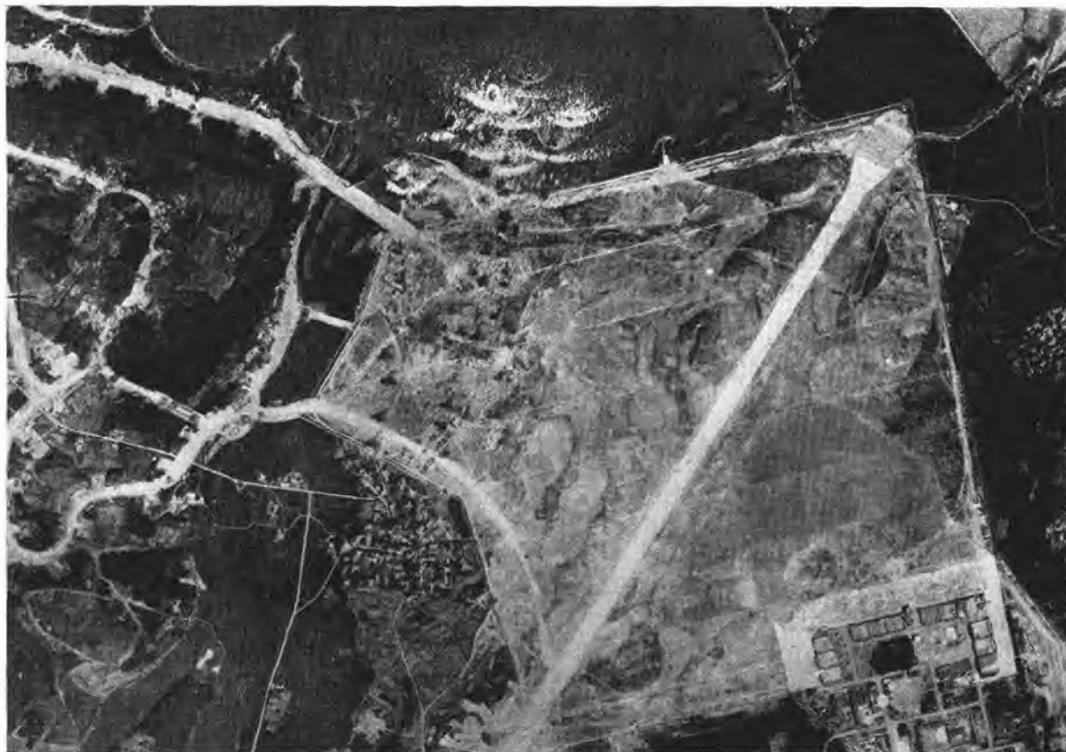
FIGURE 33. Strike photograph from bomber, illustrating fragmentation patterns obtained on air field at Tsuiki, northern Kyushu, August 8, 1945. Bombs were 260-lb fragmentation, fuzed T-50-E1, released from 10,000 ft. Some bombs burst over water, giving sharply defined fragmentation patterns (Army Air Forces photograph).
