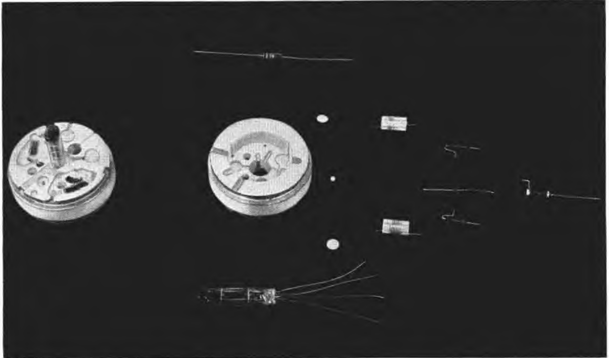
FIGURE 7. Oscillator assembly using ceramic block (Globe-Union, Inc., photograph).
