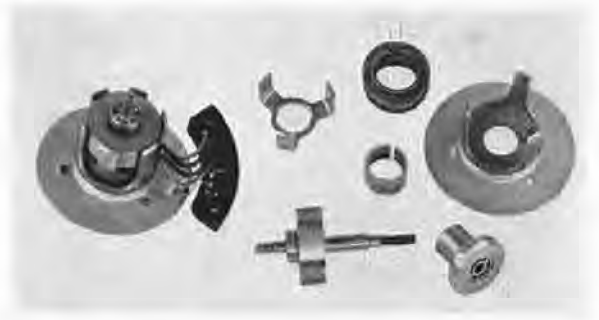
FIGURE 71. T-82 generator and principal components. Assembled generator is shown at left. Grouped at right are spider, coil, core, rotor, center stud with upper bearing, cup with cover plate.
