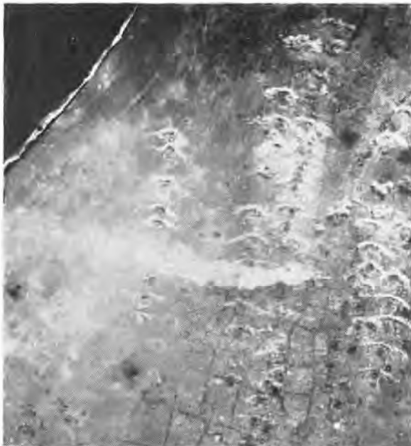
FIGURE 32. Strike photograph from bomber, illustrating fragmentation patterns obtained on beach fortification area, Iwo Jima, February 17, 1945. Patterns are from several trains of 260-lb fragmentation bombs, fuzed T-50-E1, released from 5,000 ft. (Army Air Forces photograph.)
