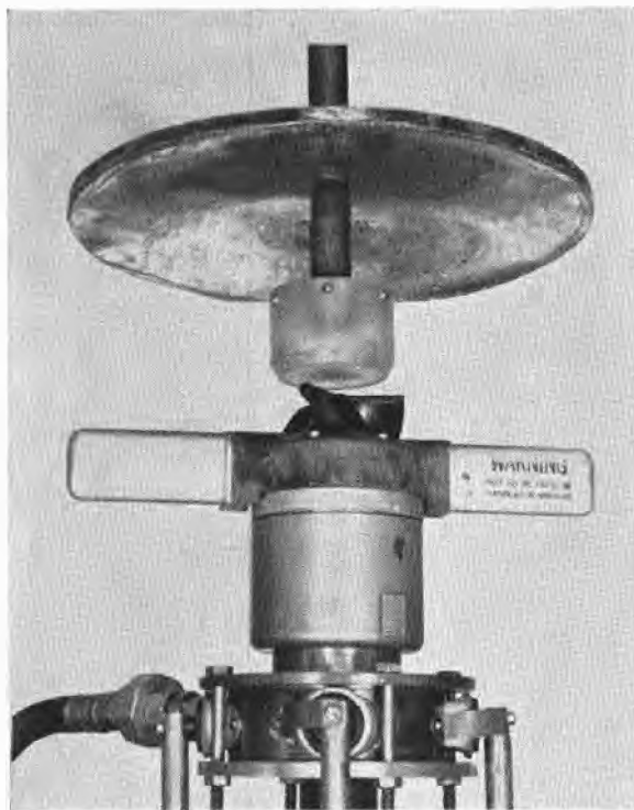
FIGURE 5. Disk load for bar-type fuzes. Central tube and nozzle carries compressed air to drive windmill.
