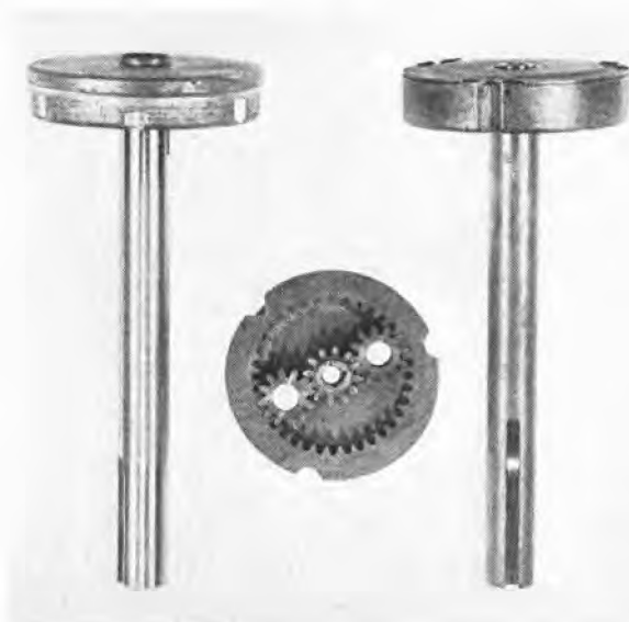
FIGURE 21. Planetary-type speed-reducing device for T-50 fuzes.
