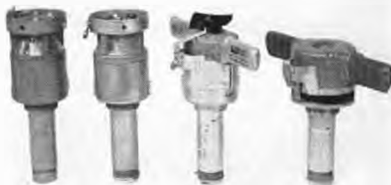
FIGURE 5. Radio proximity fuzes for bombs. These are, from left to right: (1) T-50-E1 fuze for air-to-ground use on M-30 and M-81 bombs; (2) T-91 fuze, a later and improved version of T-50-E1, for use on M-30, M-81 and M-64 bombs; (3) T-51 fuze, air-to-ground use, for use on all bombs of 100-lb size or larger; and (4) T-82 fuze for use paralleling T-51.
