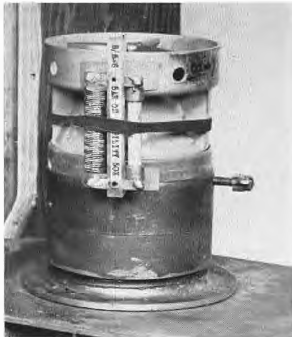
FIGURE 2. Compensated loading resistor on ring-type fuze.
