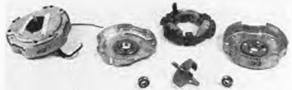
FIGURE 27. Details of generator using drawn shell construction.
