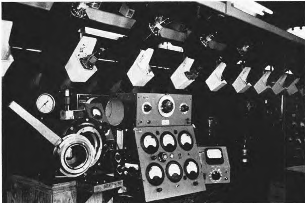
FIGURE 34. Final test position on production line. Fuzes are shown arriving at position via overhead conveyor belt (Emerson photograph).
