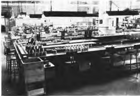
FIGURE 32. Assembly line for oscillator units. Oscillators are moved along trough shown on left side of photograph (Emerson photograph).
