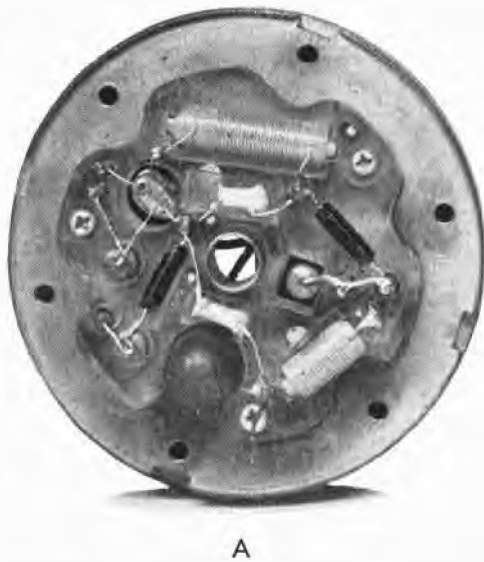
FIGURE 14. RGD circuit for T-50 fuzes. A is photograph of oscillator block. B is circuit diagram arranged to correspond to photograph.
