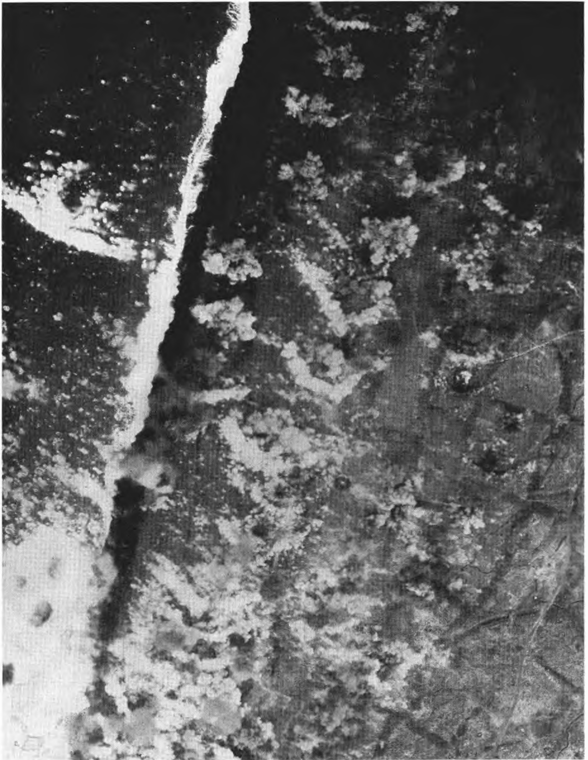
Strike photograph of the first operational use of proximity fuzed bombs. The target is the beach area of Iwo Jima during the pre-invasion bombing of the island. The characteristic crescent-shaped fragmentation patterns of air-burst bombs are clearly recognizable. (Army Air Force photograph.)
