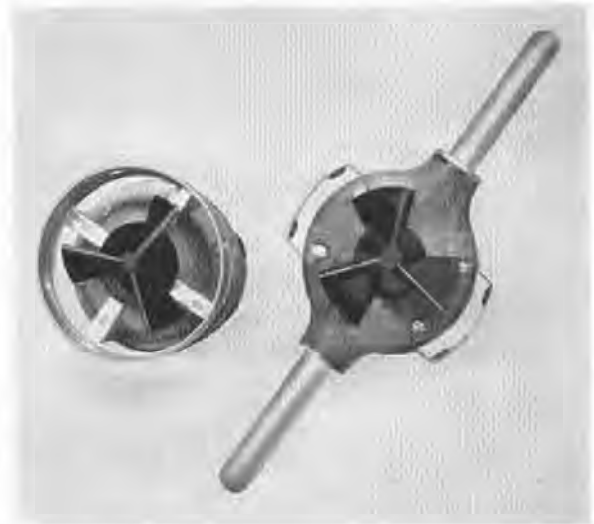
FIGURE 59. Plastic vanes on bomb fuzes. Left, T-50-E1; right, T-51.
