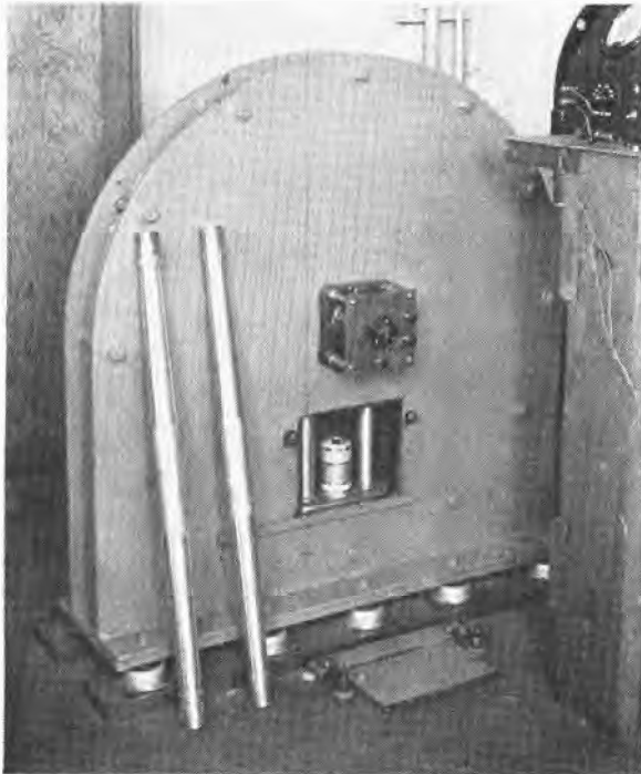
FIGURE 32. Front view of high- g centrifuge for testing mortar fuzes.
