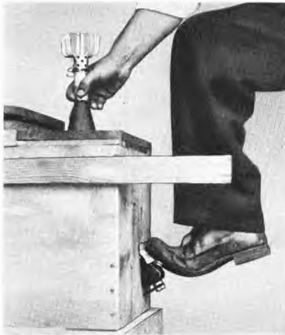
FIGURE 43. Shell being magnetized in magnetization coil.
