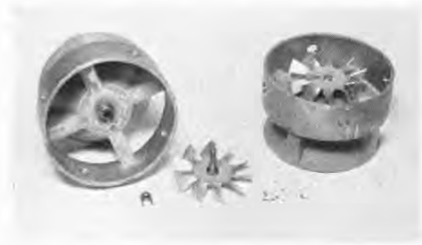
FIGURE 15. Vane and vane bearings for generator-powered bomb fuze.
