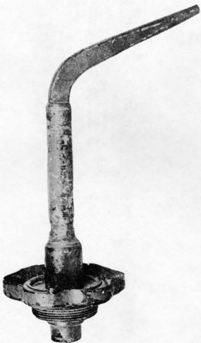
Soviet Tilt-Rod Fuze MVSh-46
