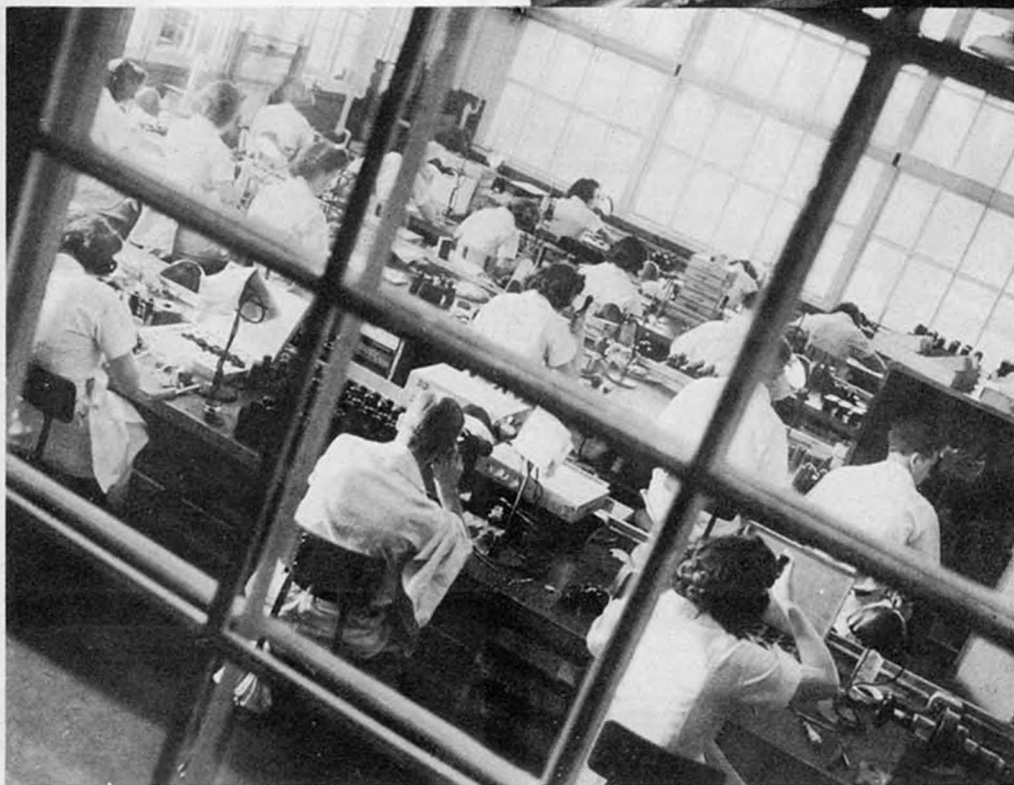
The interior optical parts of a military binocular, after final rinsing, are assembled in temperature-controlled rooms that are supplied with dust-free, filtered air.
