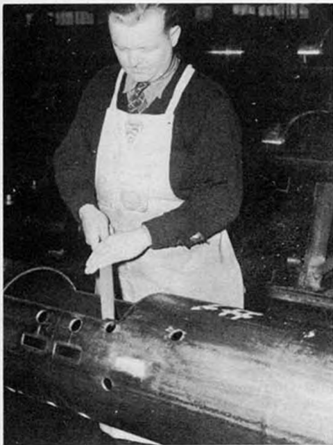
Above: Range Finders are filled with compressed gas and immersed in water to reveal leaks. Below at left: Skilled hands prepare a Range Finder
