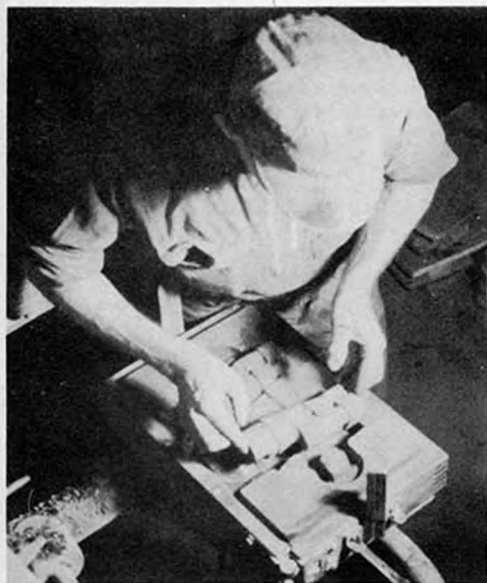
Making the Mould for a Navy Night Glass. Sand casting supplements die-casting to speed up production of this essential model.
