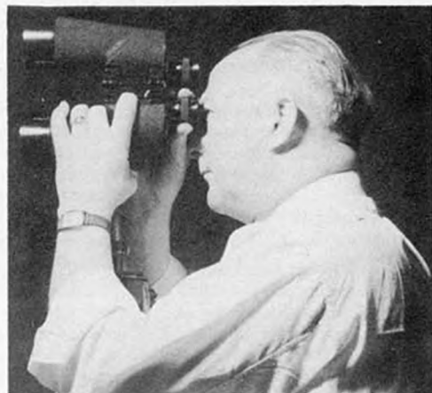
An inspector makes a final test for definition, optical performance, and resistance to shock.
