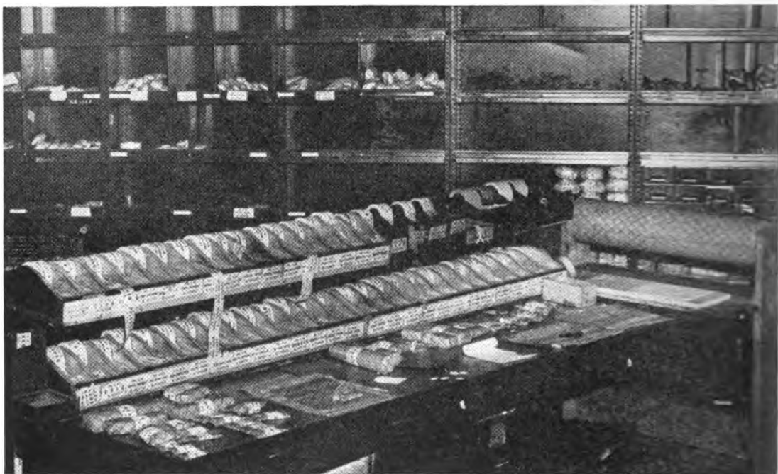
Figure 59. Scene of Interior Depot Packaging Line Showing Materials and Imprinted Pressure-Sensitive Tape for Identification of Packages.
