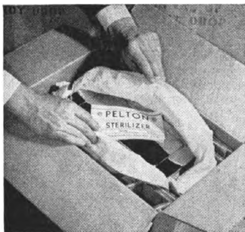
Sterilizer cabinet wrapped in creped cellulose wadding to prevent damage to the polished surfaces. Corrugated board cells are used to float the cabinet in the container.
