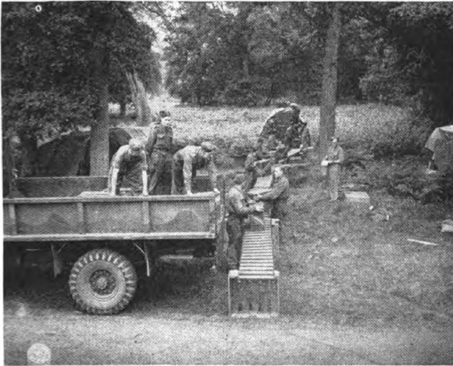
Figure 23. Use of Roller Conveyor in Communications Zone Depot—Typical of Labor Saving Expedients Often Used in Such Installations.
