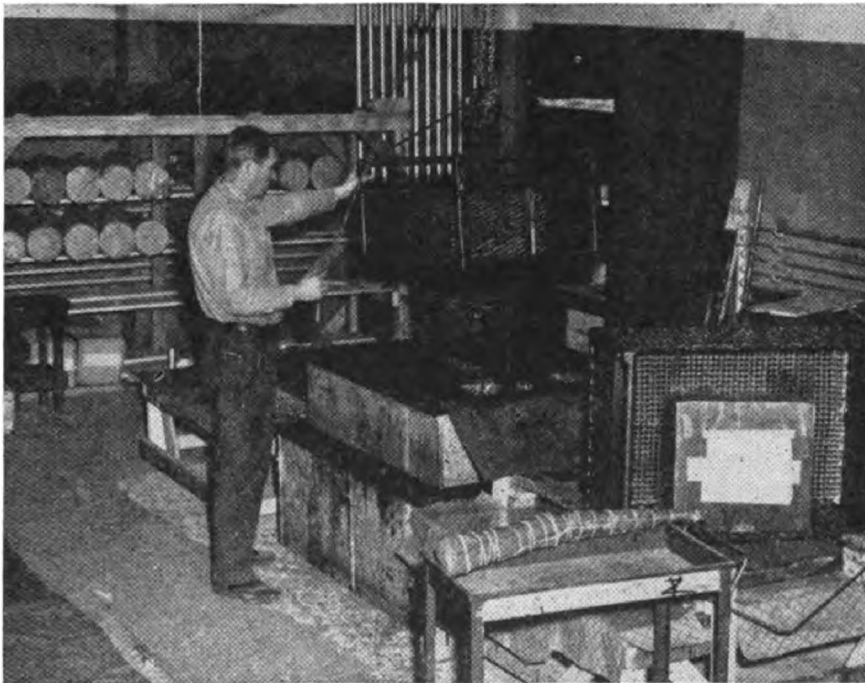
Scene of interior depot packaging line, showing Method IA packaging. Preserved parts have been wrapped in grade C material, and are awaiting immersion in wax sealing compound.
