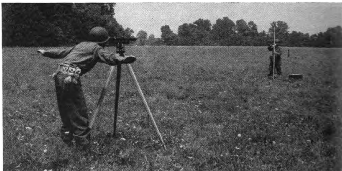
Figure 34. Determining the Relative Heights of the "Sky-Screens," and Gun Muzzle by Means of an Engineer's Level.
