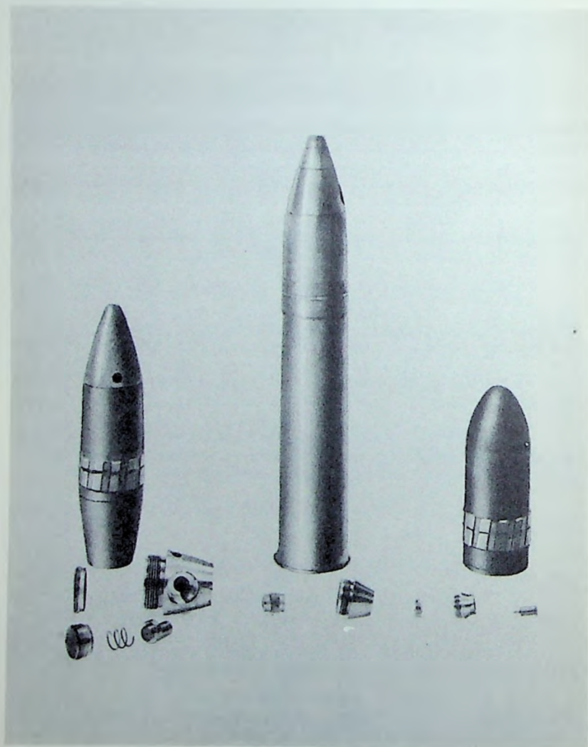
FIGURE 38. - THE AMMUNITION FOR THE 37-MM GUN, M4.
