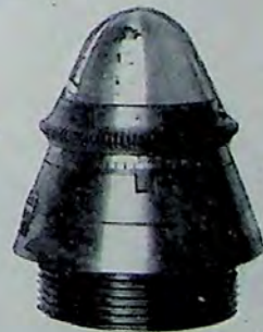
Fig. 290 Type 91 Time (with setting ring)
