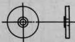
328773-24 INSULATOR USE: UNDER "LIVE" TERMINAL AT FRONT OF RACK
