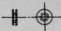
328773-28 BUSHING USE: FITS IN LOOP OF MANUAL CONTROL CABLES AT TOP OF RACK
