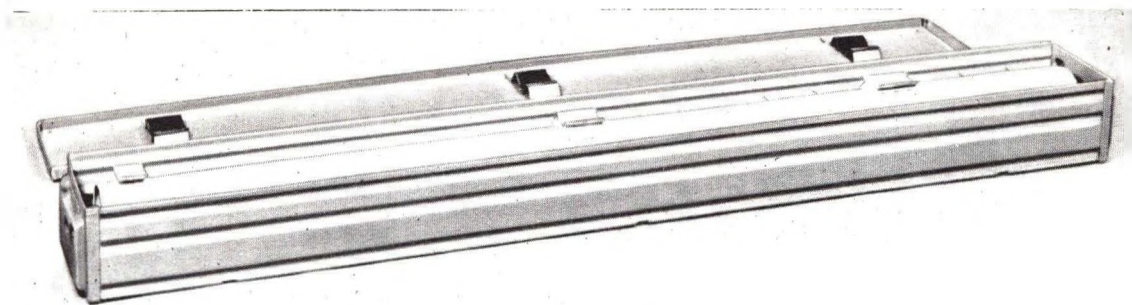
Figure 4-7. Motor Container (With Motor Ready to Ship).
