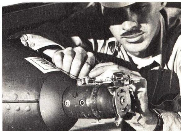
Figure 4-11. Safety Wire Removed.
