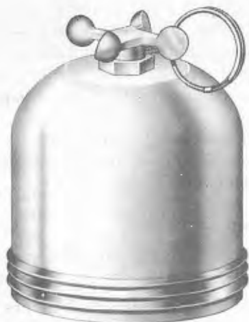
Figure 2-41.—Multi-Position Fuze AN-M173A1, Installed in Igniter M23.
