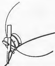
THREAD ARMING WIRE THROUGH FUZE EYELET HOLES. ATTACH SAFETY CLIP. REMOVE COTTER PIN.
