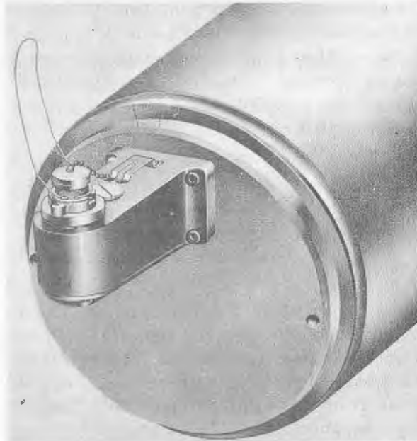
Figure 11-56.—Weapon Connector Mk 22 Mod 0, Installed.
