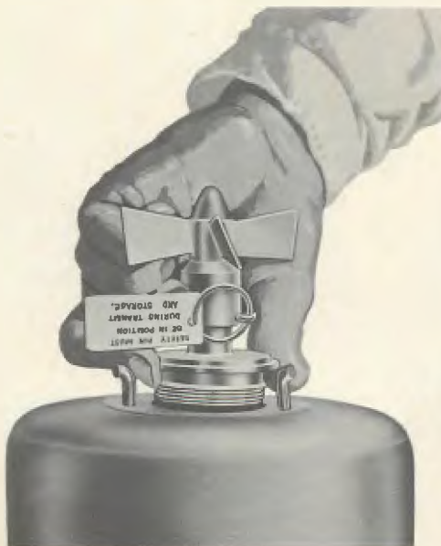
Figure 6.4—Starting Nose Fuze into Rocket Head.
