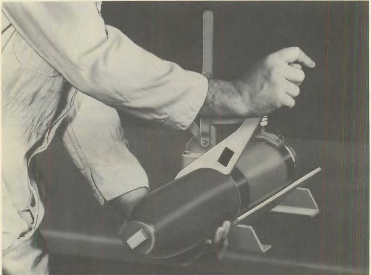
Figure 6.10—Use of Spanner Wrench in Assembly of 5.0-Inch Head and Motor.
