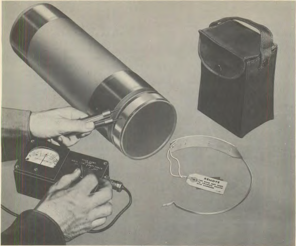
Figure 7.3—Testing of a 5.0-Inch Rocket Motor Igniter Circuit with Circuit Continuity Tester Model 680A.
