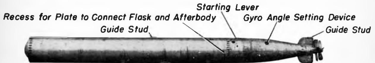
Figure 30—Type 6th year torpedo with warhead removed.
