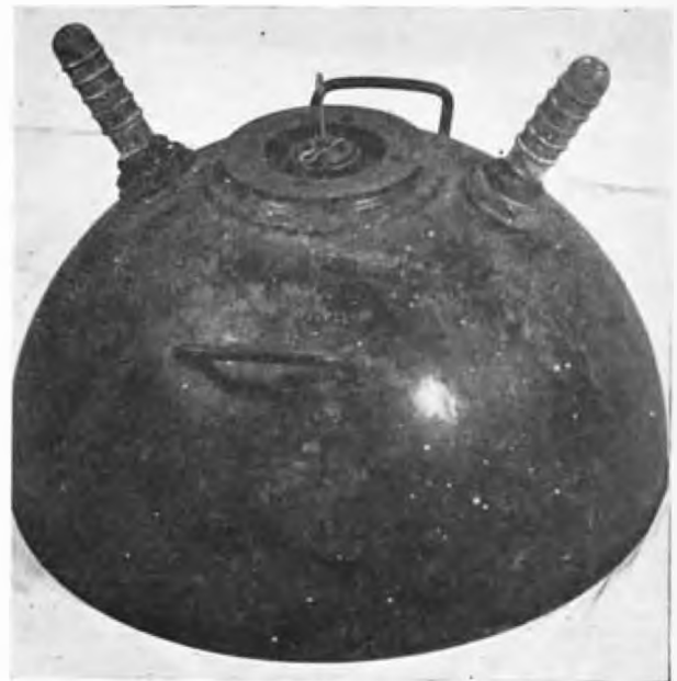
Figure 14—The JE mine. Note the safety fork in place.
