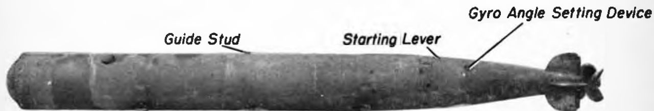
Figure 29—Type 44 torpedo with warhead removed.
