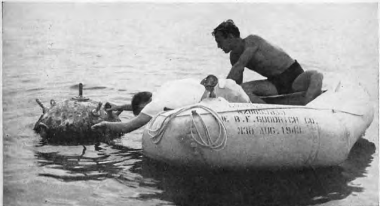
Figure 7—The JB Modification 3 Model 1 floating. Note the horn in the cover plate.
