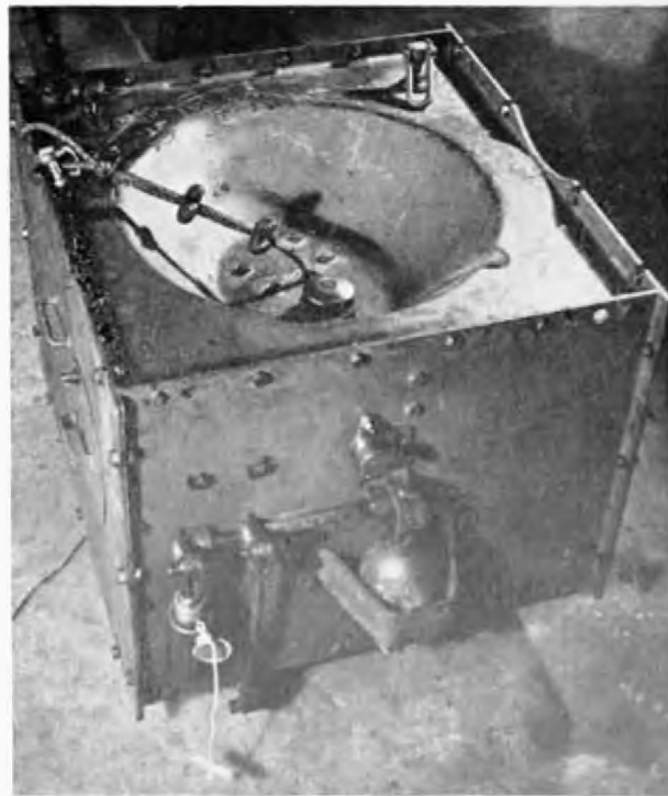
Figure 5—JB mine anchor. The same anchor is suitable for any of the various JB types.
