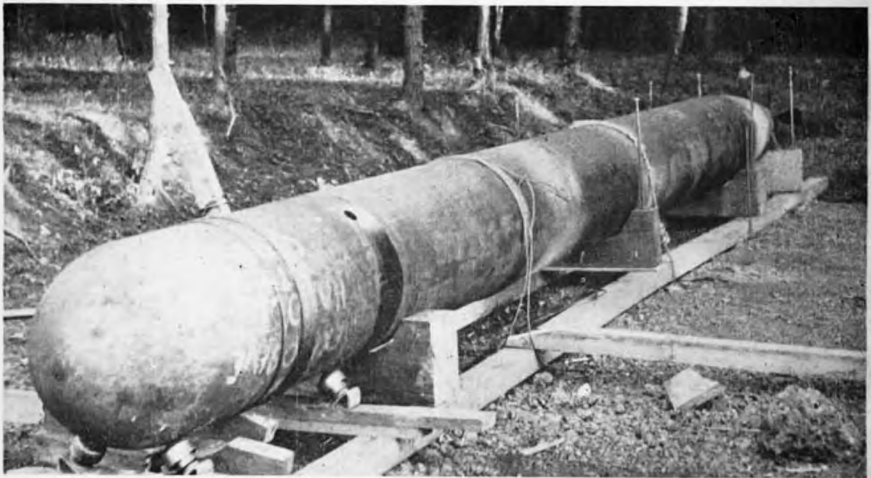
Figure 36—This 24-inch destroyer or cruiser launched torpedo is one of the largest underwater ordnance items used by the Japanese. Its use of oxygen instead of compressed air allows it to travel with practically no visible wake.
