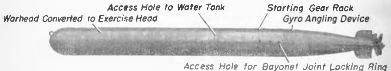
Figure 33—The aircraft and PT boat launched Type 91 torpedo.
