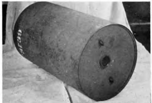
Figure 28—Two views of the Type 95 depth charge. Note the bolted end plate.
