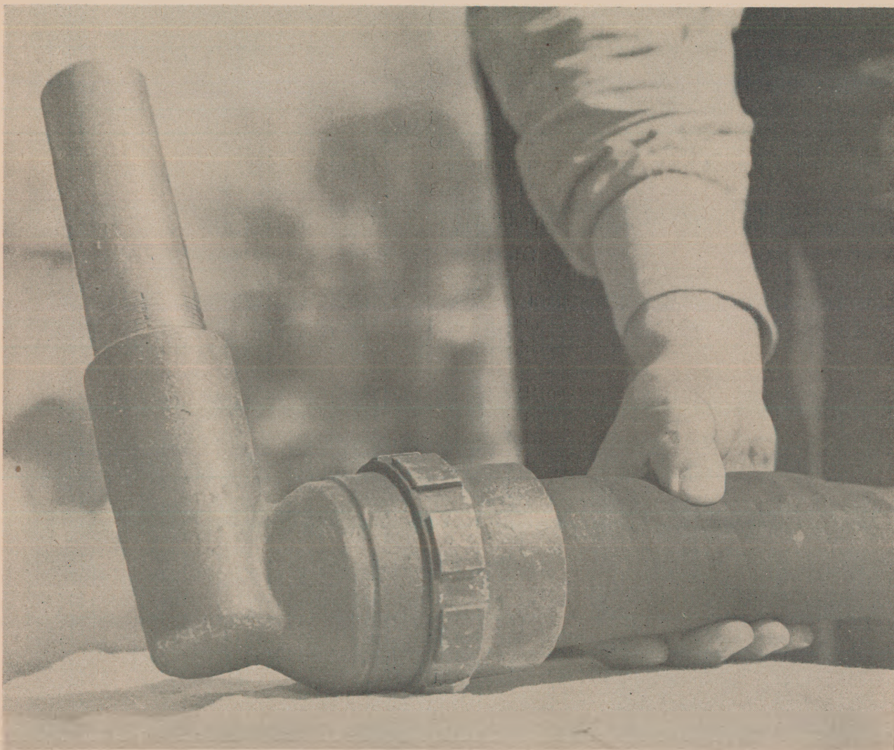
Figure 18—Adjustable nozzle for Incendiary Mixer Mark 1 Mod 1. Note calibrations. The desired 6 \pm \frac{1}{2}\% intake of Type 1 Napalm is usually attained by setting the nozzle on or slightly below "4".
