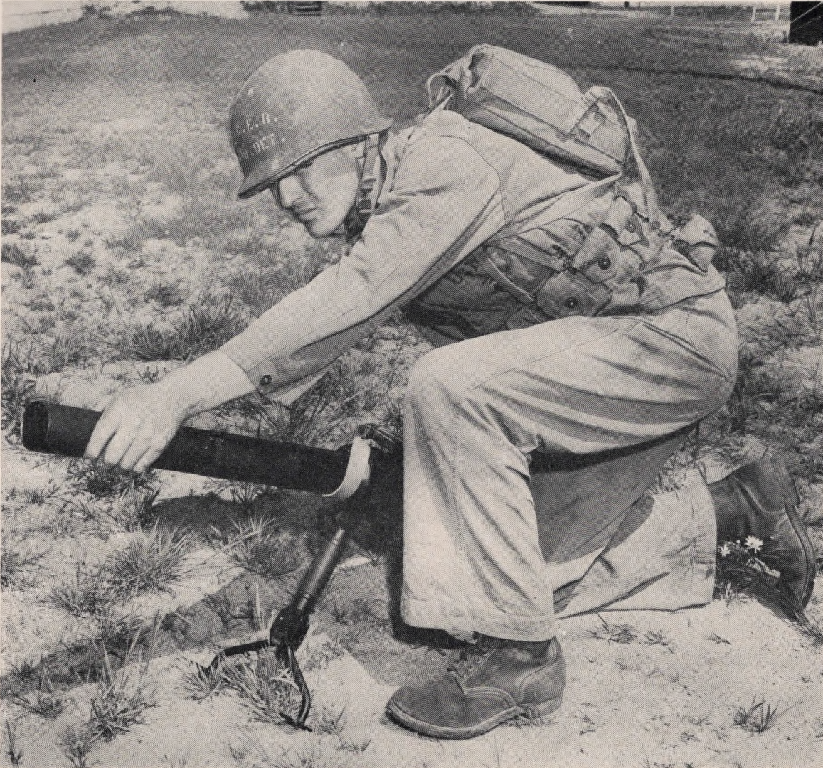
Figure 3.—The cocking position. With the butt held firmly to the ground, grasp the barrel with the left hand and pull it rearward until the sear engages the front of the piston with a distinct click.
