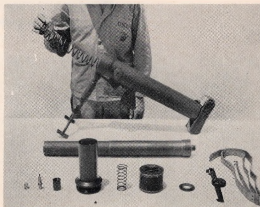
Figure 20.—Step 12—Remove the recoil spring.
