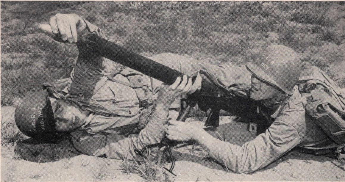
Figure 6.—Loading from prone position. The gunner elevates the barrel of the shoulder mortar as the loader inserts the shell.
