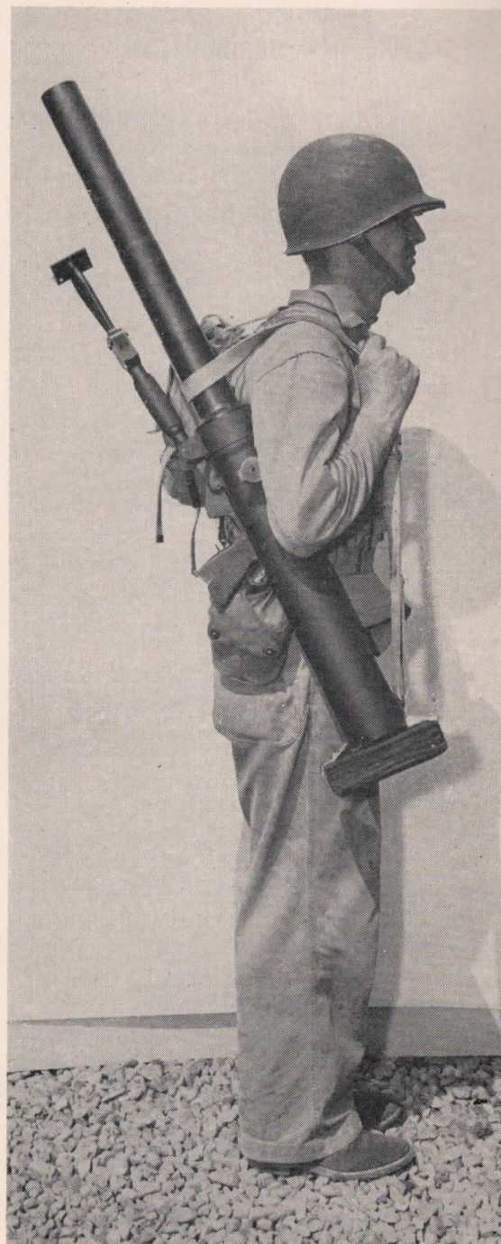
Figure 2.—The Garrett 60 mm Shoulder Mortar Mk 1 Mod 0 in carrying position with monopod folded beneath barrel.
