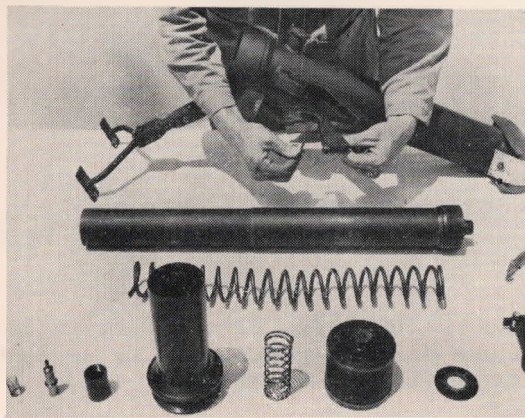
Figure 19.—Step 11—Remove the trigger hinge pin, trigger and trigger spring. The safety disconnect is disassembled by removing the disconnect pin, disconnect slide, disconnect, disconnect spring and disconnect cover.
