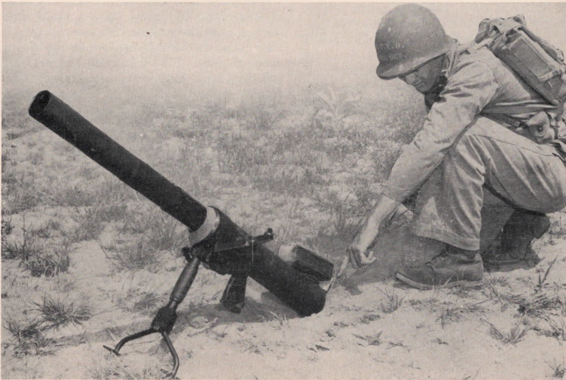
Figure 7.—Shoulder mortar in high angle firing position. Note the butt is well seated in the ground.
