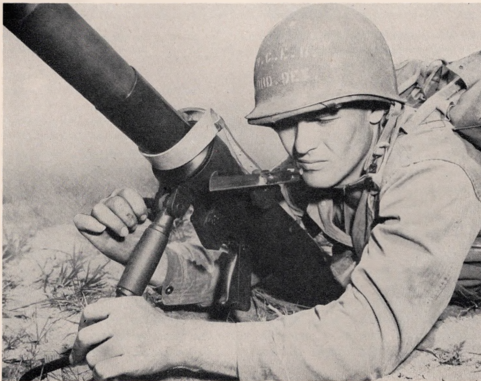
Figure 4.—After the sight has been aligned on the target, cross leveling is accomplished by rotating the shoulder mortar until the bubble is centered.
