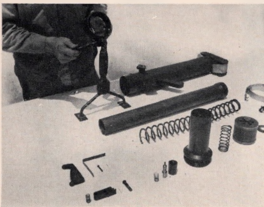
Figure 21.—Step 13—Remove the monopod hinge collar from the recoil spring housing. The monopod is removed from the collar by unscrewing the adjusting clamp.
