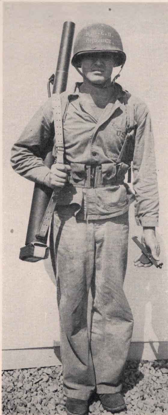
Figure 1.—The Garrett 60 mm Shoulder Mortar Mk 1 Mod 0 in carrying position. Sight has been removed preparatory to placing it in its carrying case attached to a rear pocket of the cartridge belt.
