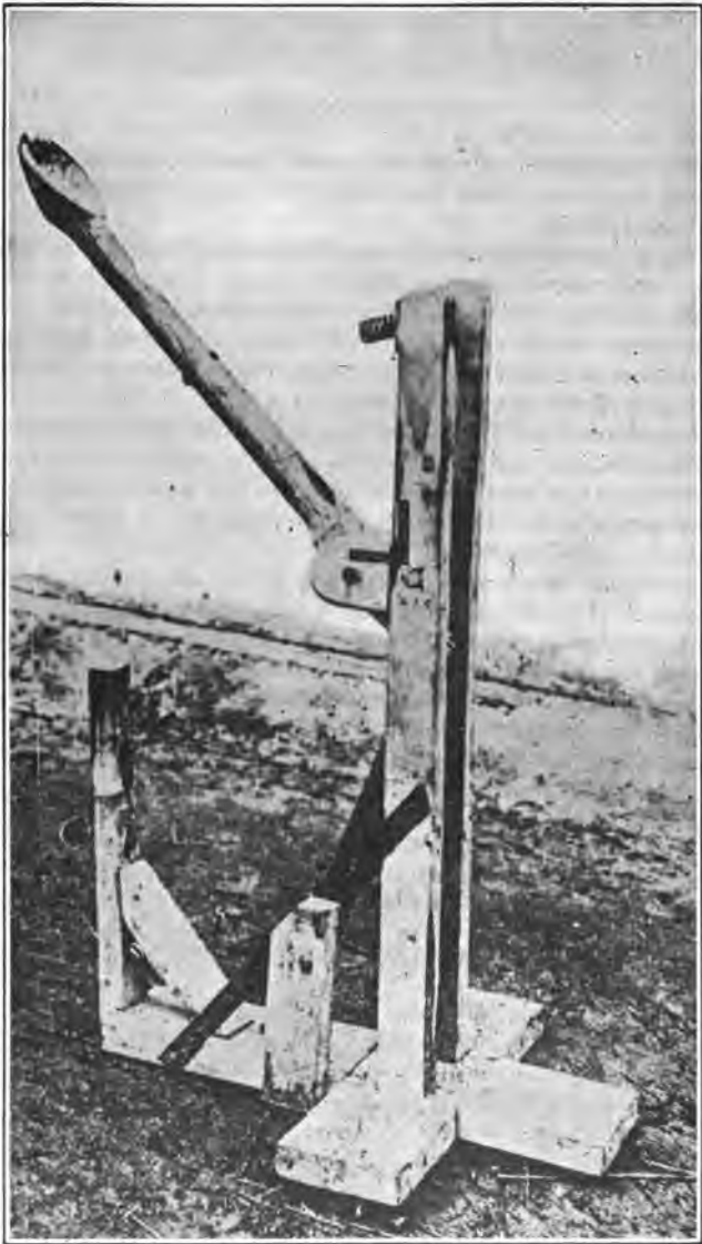
FIG. 15.—THIS DEVICE FOR CASTING GRENADES OR BOMBS IS OF VERY ANCIENT DESIGN, BUT IS BEING USED EFFECTIVELY FOR DROPPING BOMBS ON HOSTILE TRENCHES IN THE EUROPEAN WAR.
