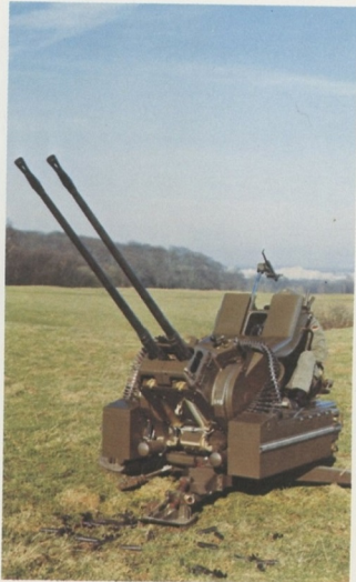
Twin Rheinmetall MK20-RH 202 A.A. System firing break-up cartridges
