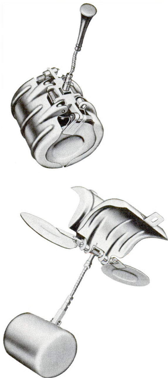
Figure 11-6.—The 4-pound Fragmentation Bomb AN-M83 (closed and open).
