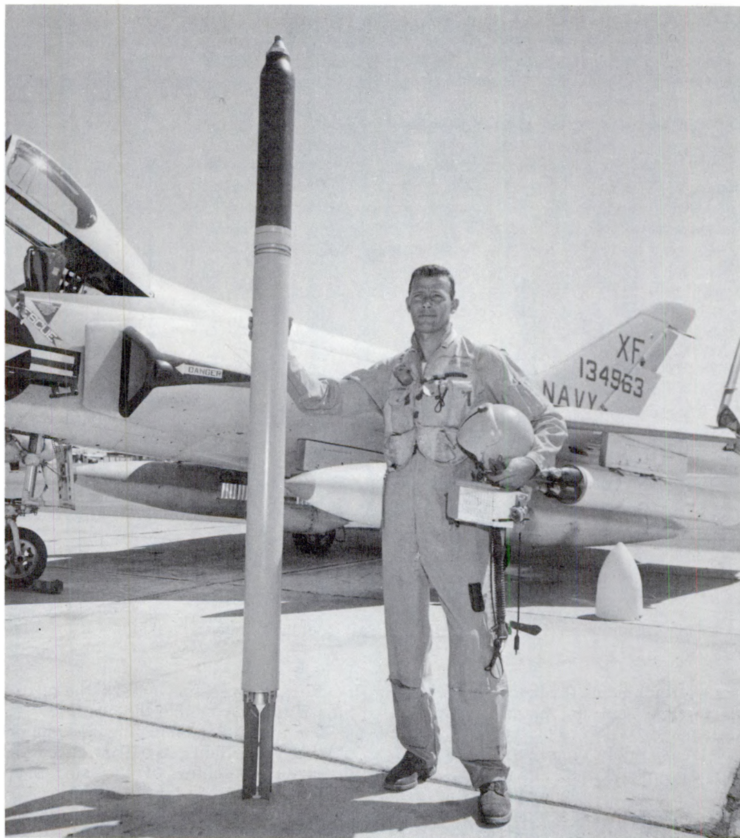
Figure 10-12.—The 5.0-inch Zuni folding-fin rocket.
