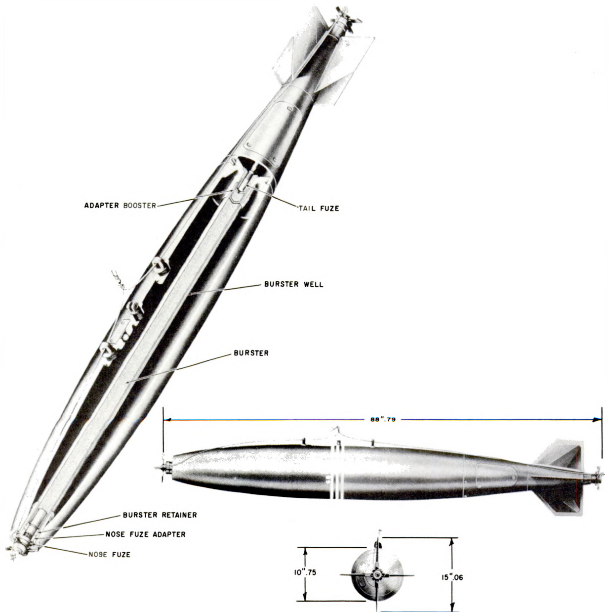
Figure 11-13. -500-Pound Chemical (Gas) Bomb Mk 94 Mod 0, cutaway view.
