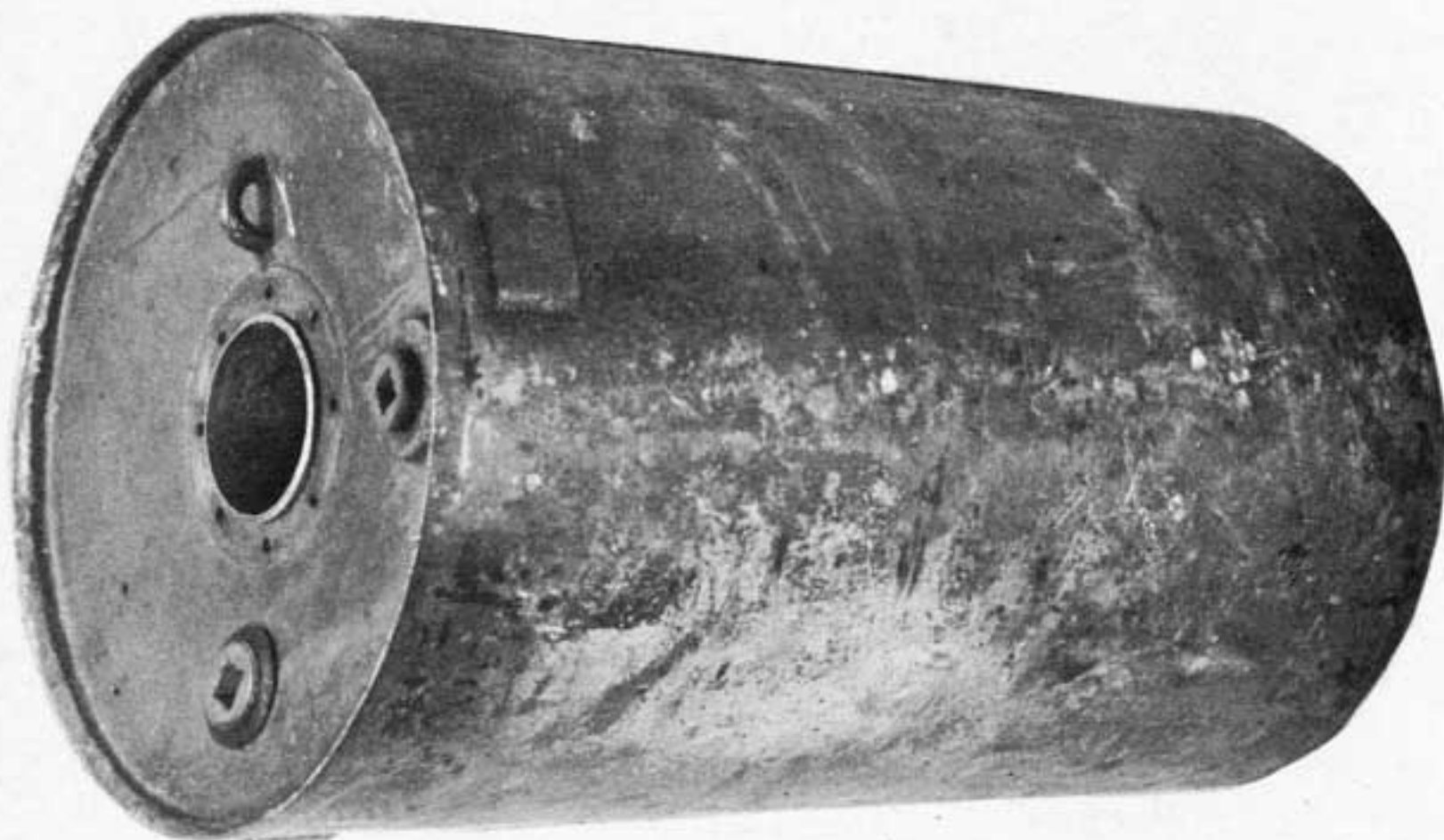
Fig. 2 - Depth Charge, Pistol End
