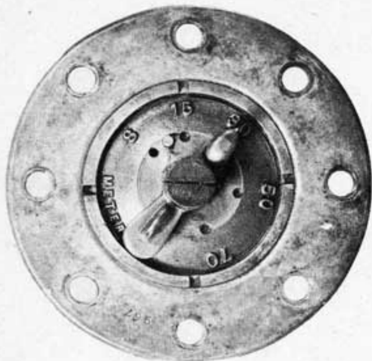
Fig. 3 - Depth Charge Pistol, Dial Setting Face
