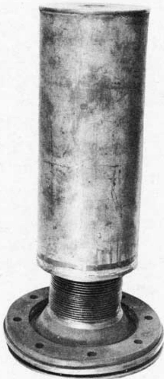
Fig. 6 - Depth Charge Booster Extender and Booster
