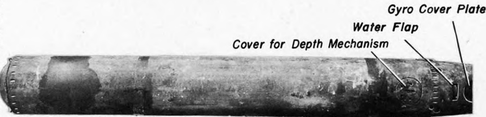
Fig. 46 - Torpedo Type 44 Mark 2 Mod 1, Flask Section, Bottom View.
