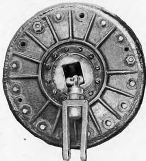
Fig. 59 - Mine Mk 6 Model 2, Base Plate, External View
