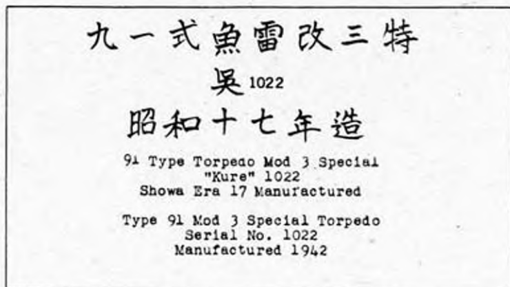
Fig.15- Type 91 Mod 3 Special Torpedo, Label on Forward End of Airflask.
