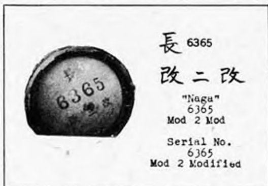
Fig. 10 - Type 91 Mod 2 Torpedo, Label on Airflask Bulkhead.
