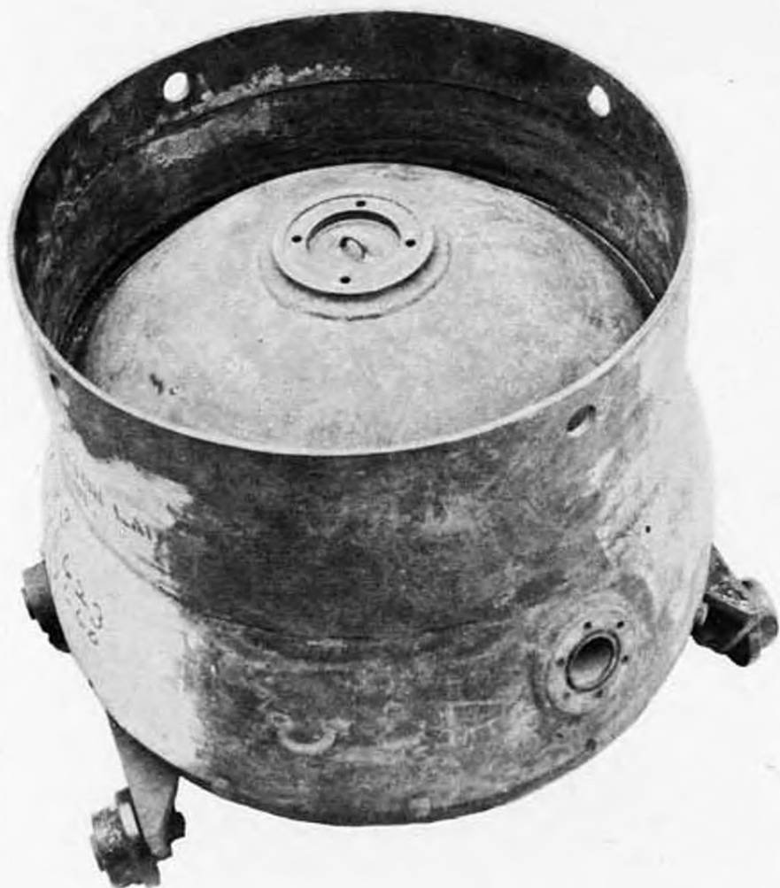
Fig. 31-- Mine Type JF (Booster Assembly Removed)
