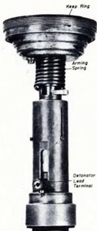
Fig. 15-- Arming Switch Detail, Mine Type JC
