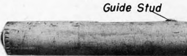
Fig. 55 - Torpedo Eighth Year Type Mark 2 Mod 2, Warhead Removed
