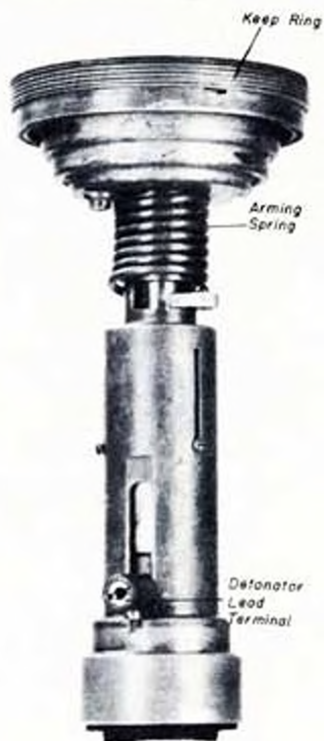
Fig. 39-- Arming Switch Detail, Mine Type JH
