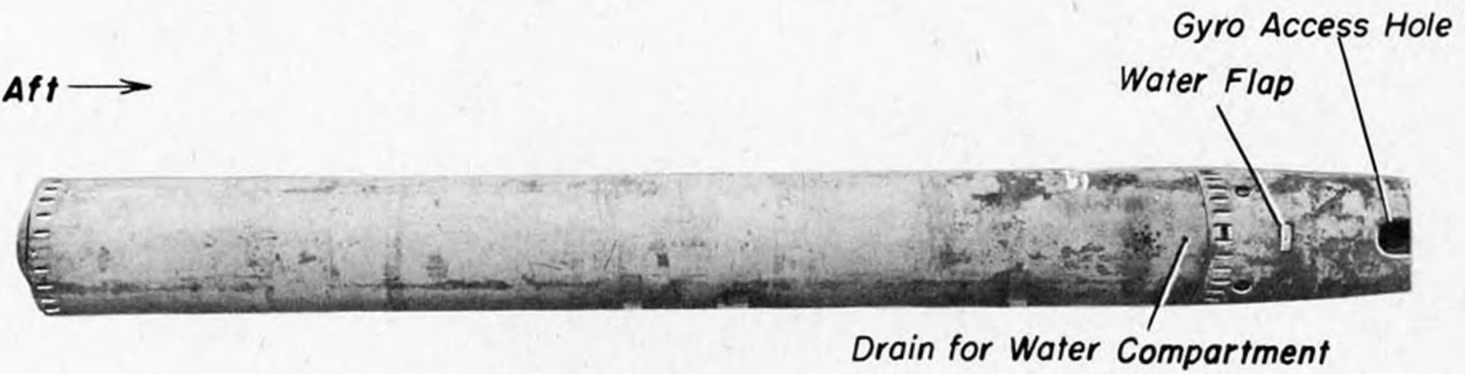
Fig. 57 - Torpedo Eighth Year Type Mark 2 Mod 2, Flask Section, Bottom View
