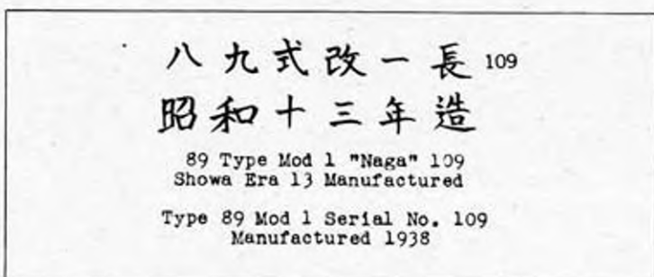
Fig.13- Type 89 Mod 1 Torpedo, Label on Forward End of Airflask, Top Centerline.
