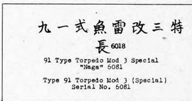
Fig. 16 - Type 91 Mod 3 Torpedo, Label on Forward End of Airflask.
