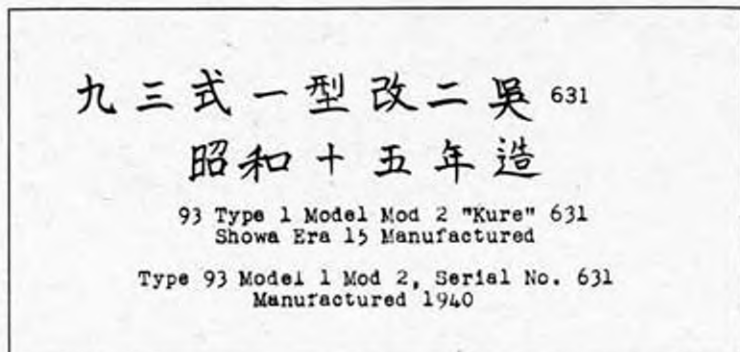
Fig.14- Type 93 Model 1 Mod 2 Torpedo, Label on Forward End of Airflask, Top Centerline.
