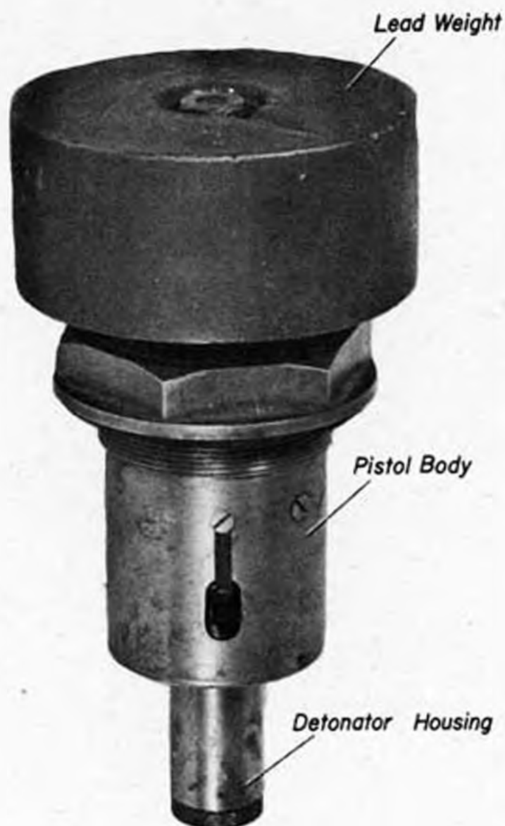
Fig. 7 - Pistol for Tactical Depth Charge.
