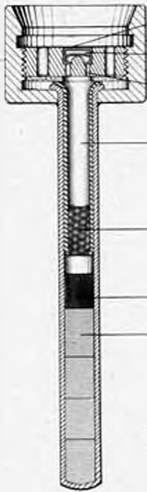
Fig. 9 - No. 49 Detonator, Mk. I, Sectional View
