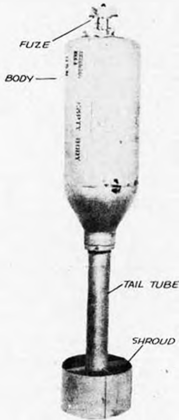
Fig. 8-- 7'2 Projector Charge (Hedgehog)
