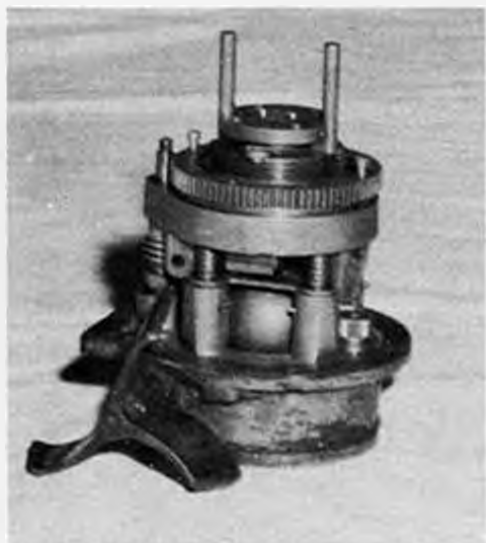
Fig. 5-- Mk. 3-2 Exploder Armed With Safety Chamber Removed
