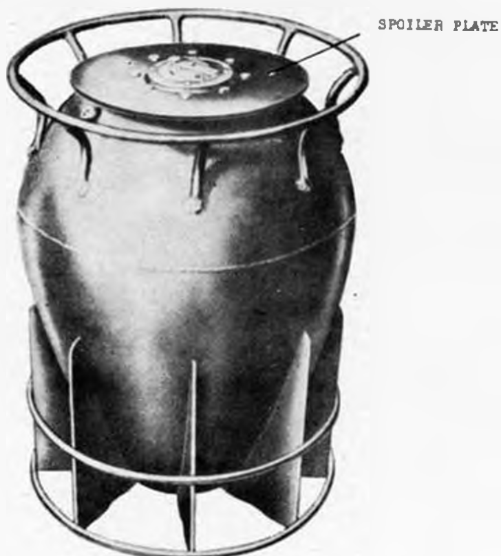
Fig. 10-- Mk. 9-2 Depth Charge with Spoiler Plate
