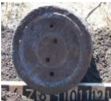
Projectile: 2.04 pounds of Explosive D. Fuze: Mk 20 Mods 0 – 2 Base Detonating Fuze Tracer: Mk 9 tracer.
