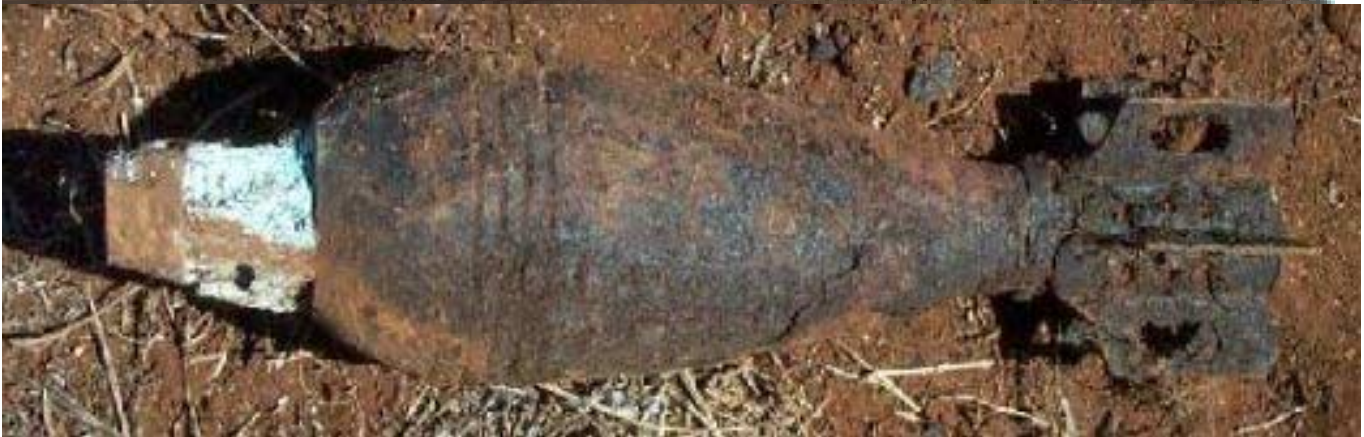
NEW of M43A1: 1.3 LBS of TNT NEW of M43A1B1: 1.3 LBS of Composition B.
