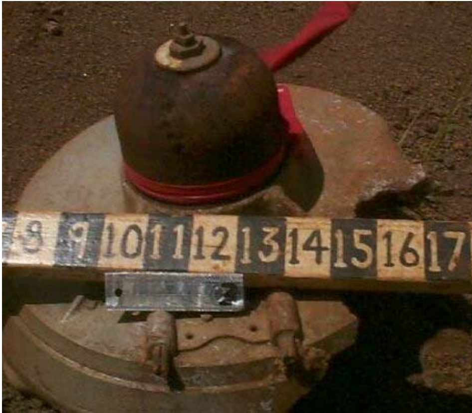
M23 Igniter still attached to the end plate of a firebomb.
