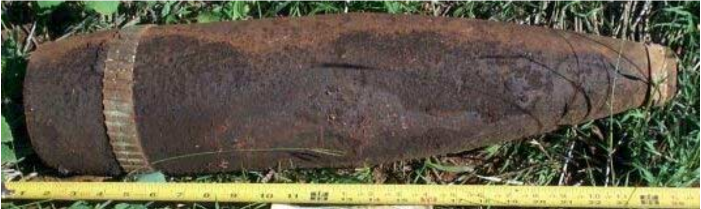
This is a spin stabilized, howitzer fired, high explosive (HE) projectile. The projectile is olive drab with yellow markings. The projectile is steel.
