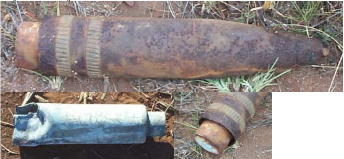
MK 48 body loaded with White Phosphorus Canister MK14.
