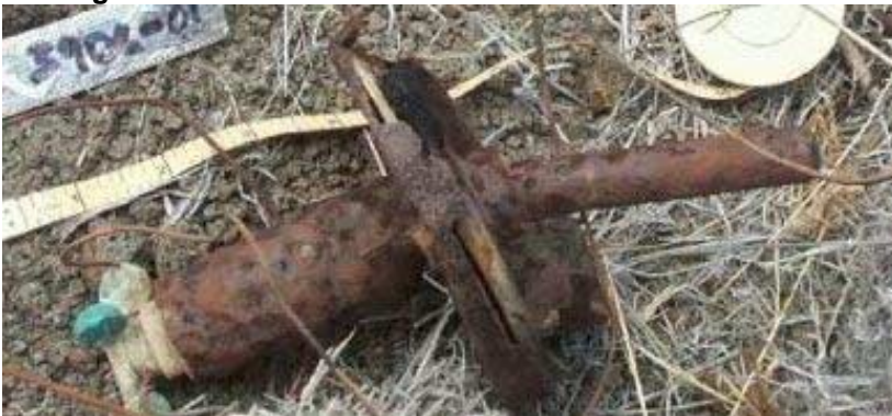
M157 Fuze with C8R1 Burster Attached
