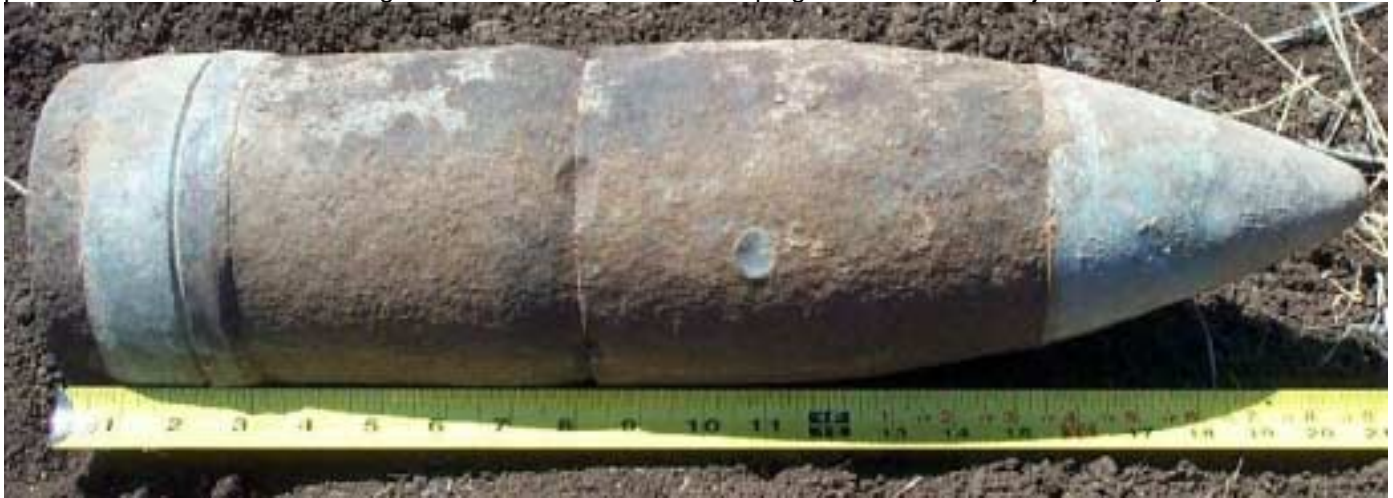
Projectile: 2.04 pounds of Explosive D. Fuze: Mk 20 Mods 0 – 2 Base Detonating Fuze Tracer: Mk 9 tracer.
