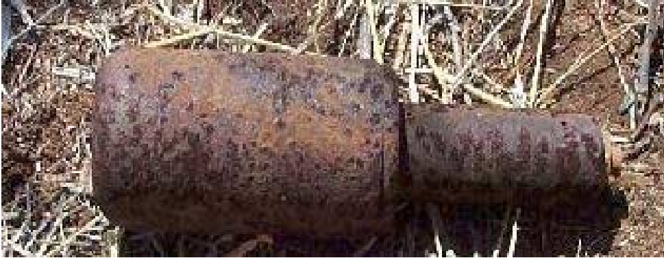
M15 External Mounted Igniter (M13 is Identical)
