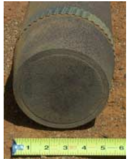
This is a spin stabilized, howitzer fired, high explosive (HE) projectile. The projectile is olive drab with yellow markings. The projectile is steel.
