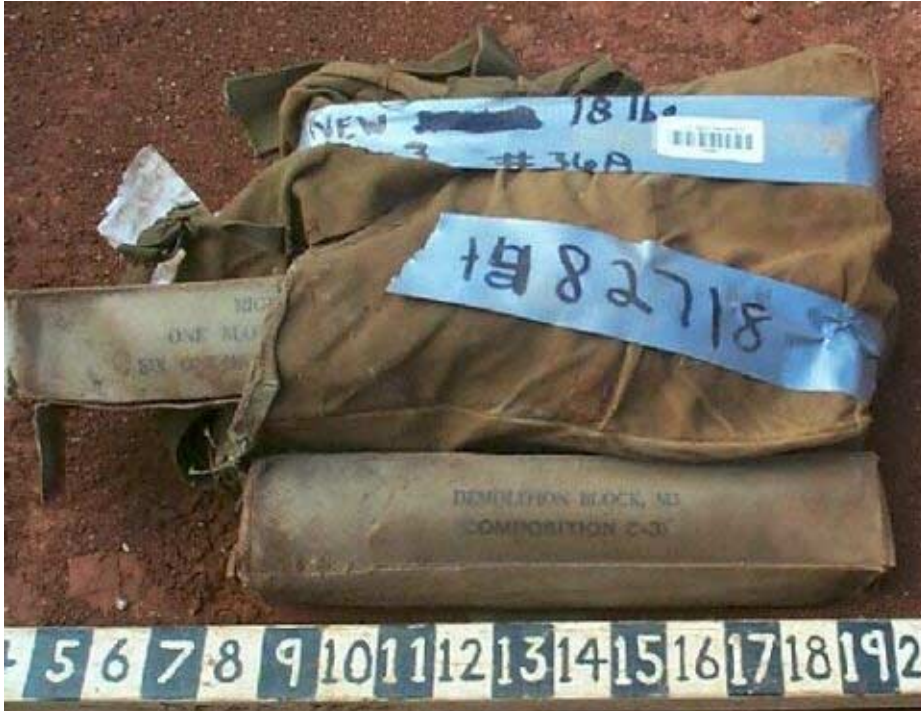
Demolition Block, M3 Composition C-3
