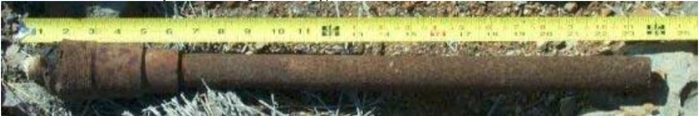
Exploder with MK219 Fuze Attached from MK4 100 LB Bomb.
