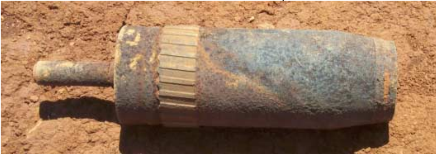
HE Projectile With MK4 Tracer. Explosives and NEW: Cast TNT .74 Lbs.
