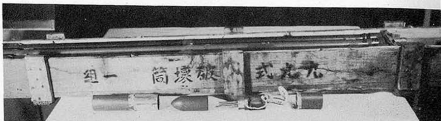
Fig. A Packing - 6 Bangalore Sections and 3 Firing Assemblies. (Assemblies in right hand compartment)
