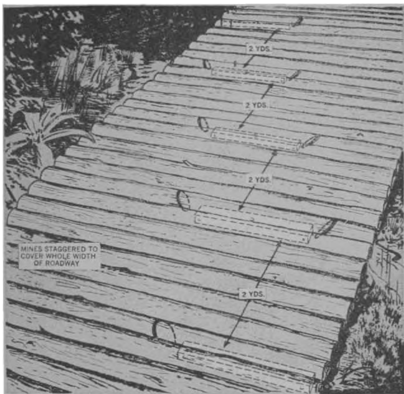
German method of laying Riegelmines under a corduroy road.
