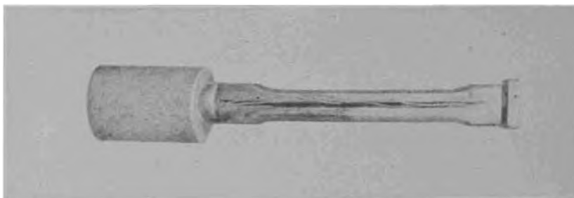
German concrete stick hand grenade, Type 2, with stick TNT embedded in the concrete.
