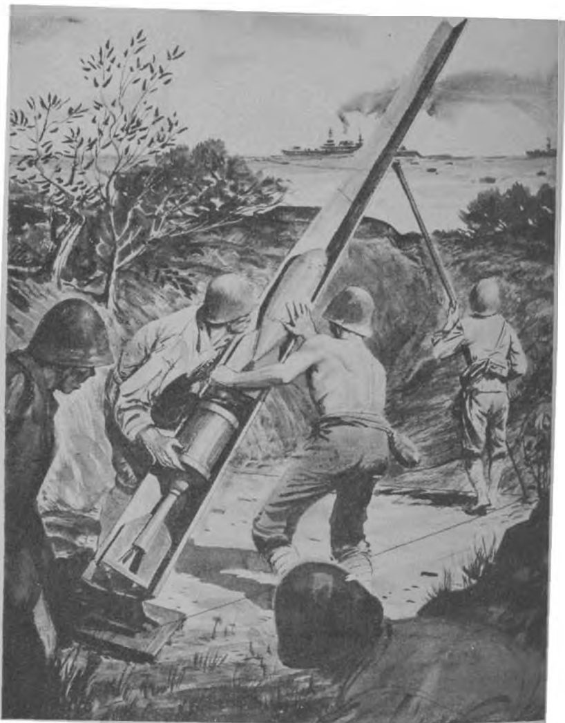
Japanese troops loading a Model 10 rocket launcher of the type captured by U. S. troops on Saipan. Only one launcher of this type has been found, and it is believed to be the result of early Jap experiments with rocket-propelled projectiles.
