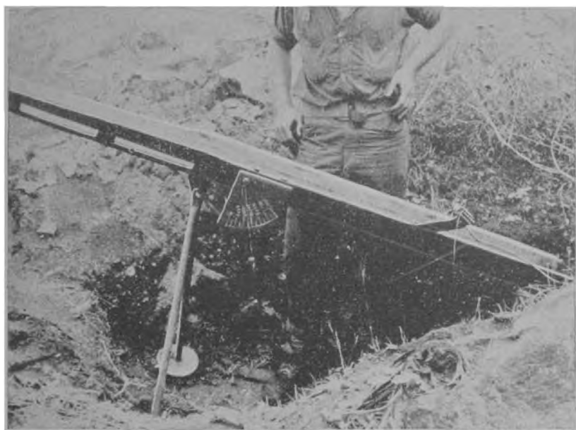
Another view of the Leyte launcher showing the forward bipod and the graduated scale of the crude ranging device.
