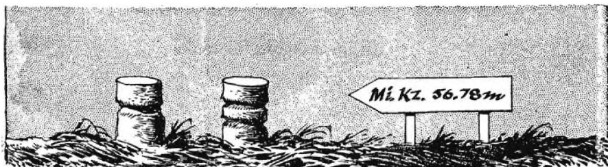
Guides to Corner, Survey, and Fix Points.
