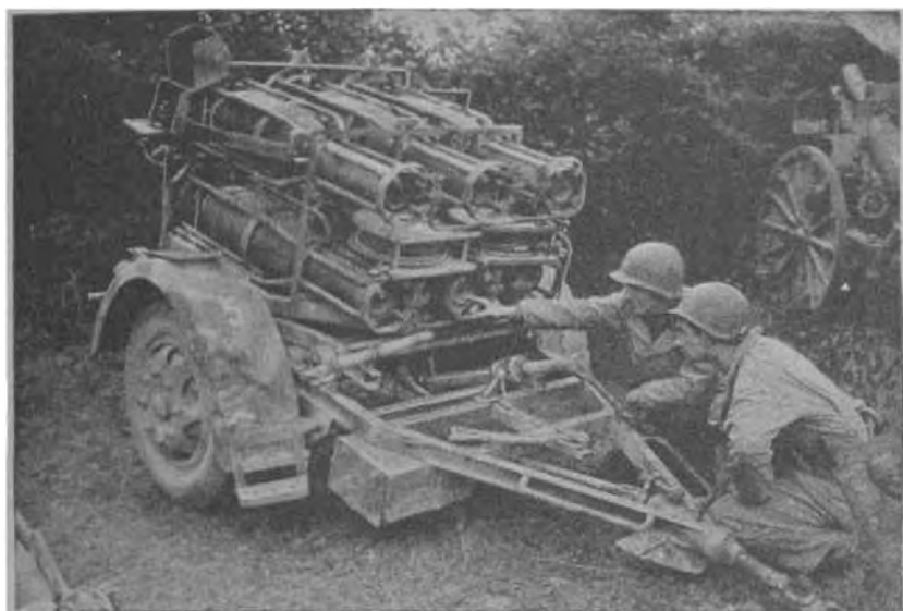
U. S. soldiers inspect a captured 28/32-cm Nebelwerfer 41. The weapon is loaded, but electrical leads are not connected to the bases of the rocket motors. Note the box (shown open) which protects the sight.
