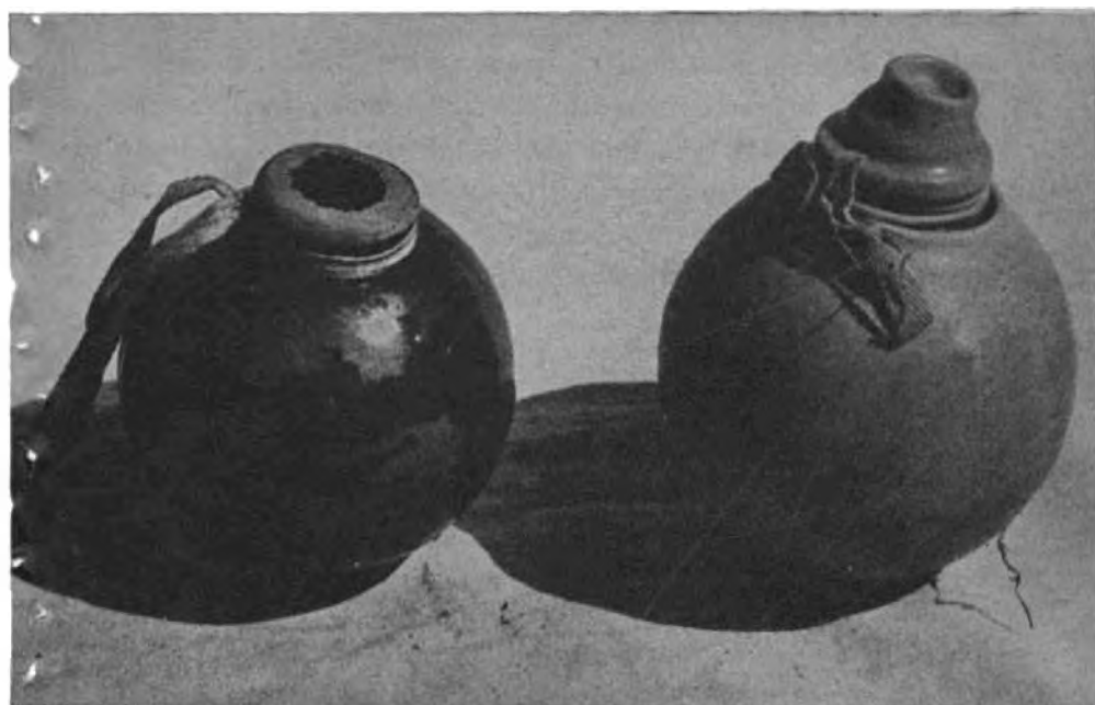
Two views of the Ceramic Hand Grenade showing (left) the grenade with carrying tape and exposed match-head fuze, and (right) the grenade with rubber cover and rubber fuze cap.
