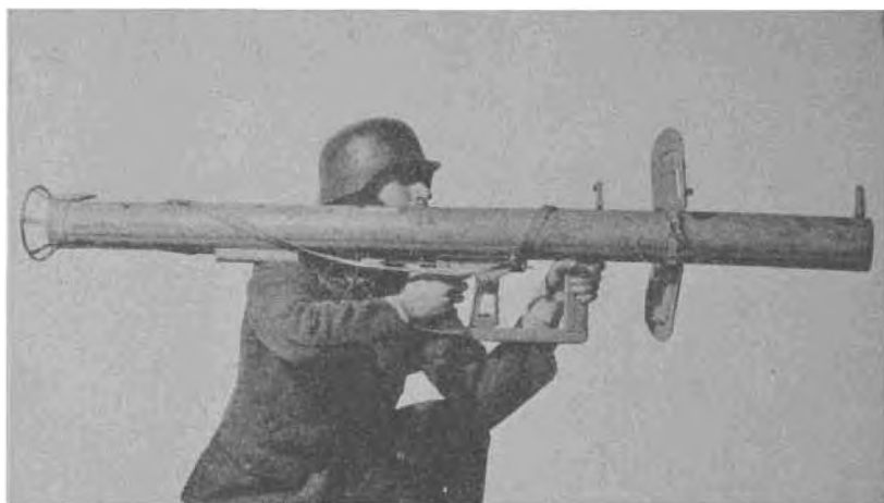
Recently captured Ofenrohr have had very noticeable fore and rear sights and shields to protect the users.
