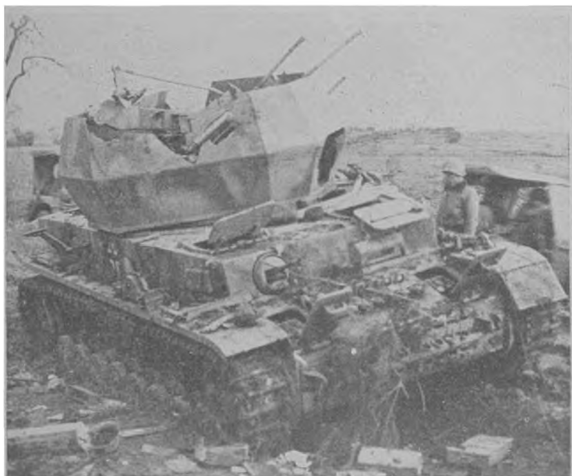
The Flakvierling 38, a four-barrelled 20-mm antiaircraft gun mounted on the Pz.Kpfw. IV chassis, is the newest version of the Flakpanzer to make its appearance with the German Army in combat.
