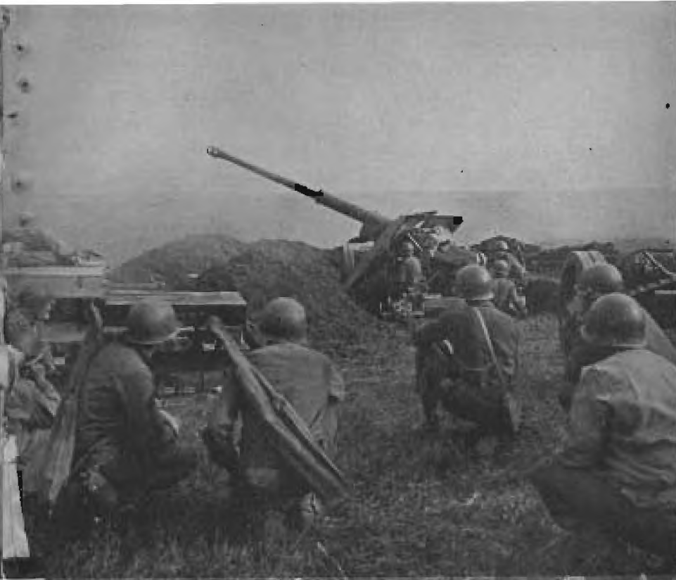
American artillerymen fire a captured Pak 43 at the retreating German army in the area around Metz, France. Ordnance Intelligence Teams often are able to repair weapons damaged by a retreating enemy and turn the guns against the former owners.
